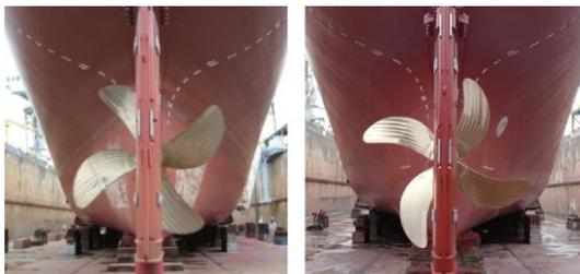
Figure 3. Minimized blade area propeller (right side)<sup>5)6)</sup>
