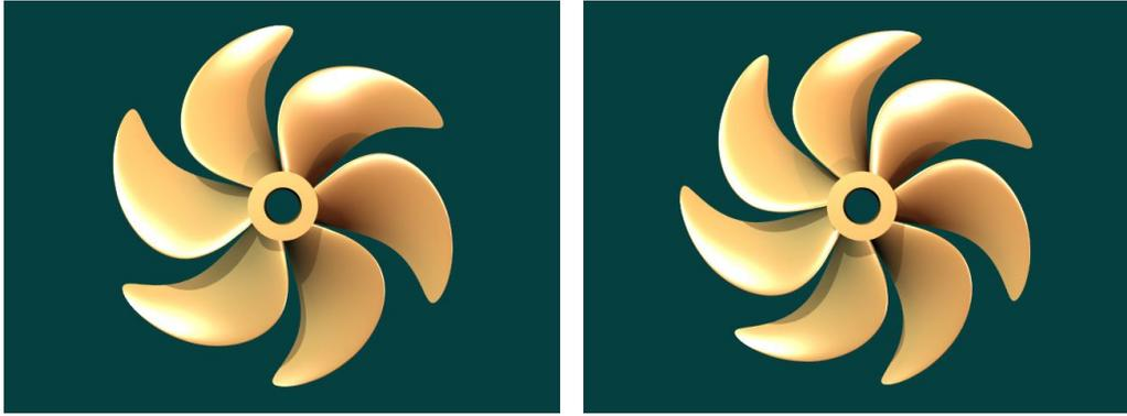
**Figure 7.** Propeller profile of 6- and 7-bladed for ro-ro ship
