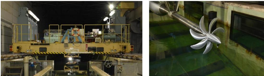
**Figure 6.** Measurement equipment for propeller open characteristics<sup>8)</sup>
