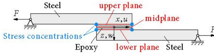
Figure 2: Considered single-lap joint under tensile loading
