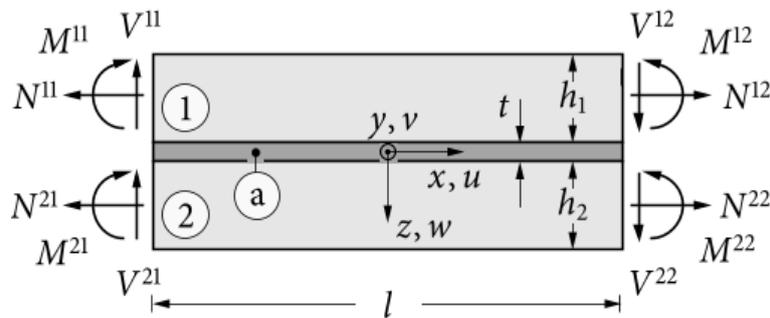
Figure 1: General sandwich-type model with geometric dimensions and applied loading
