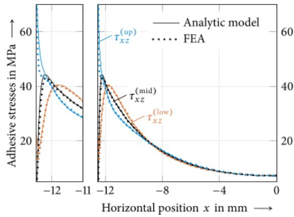
Figure 3: Shear stress distributions calculated along the centerline and the upper and lower interfaces
