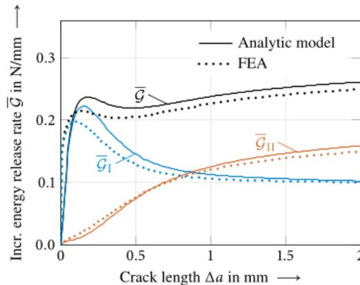
**Figure 6:** Energy release rate of the analytical and numerical model for steel adherends connected with adhesive layer of AV138 under a tensile load of 8kN
