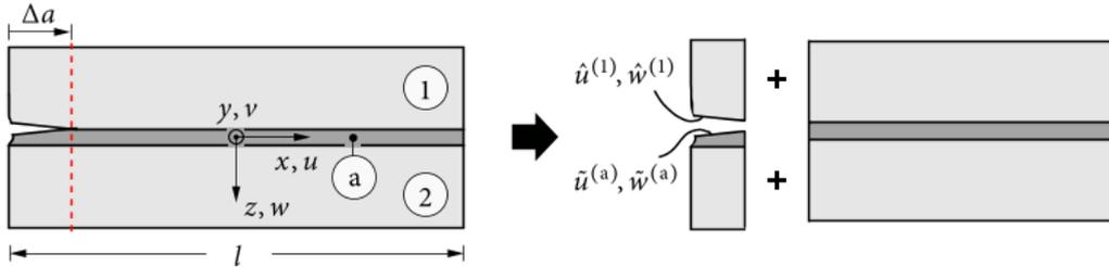
**Figure 5:** Subdivision of the adhesive joint into cracked and uncracked parts
