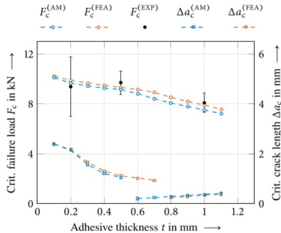
**Figure 7:** Mechanical failure loads and crack lengths for different adhesive thicknesses  $t$  according to analytical model (AM) in comparison with finite element analyses (FEA) and experimental findings (EXP) of [13]
