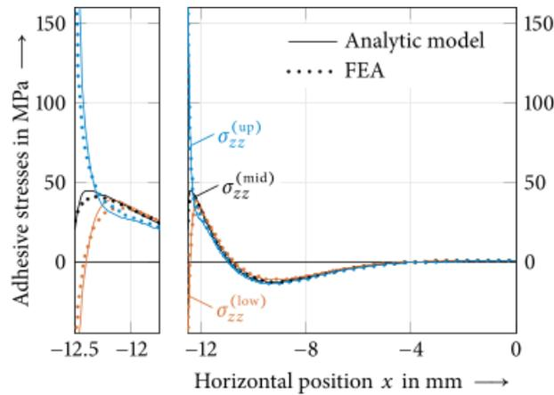
Figure 4: Peel stress distributions along the centerline and the upper and lower interfaces
