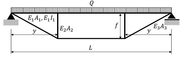
Figure 6: Beam string structure with two struts
