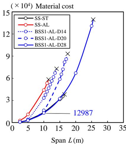
Figure 8: Material cost of BSSs with a strut versus span
