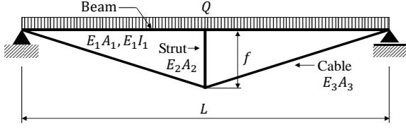
Figure 5: Beam string structure with a strut
