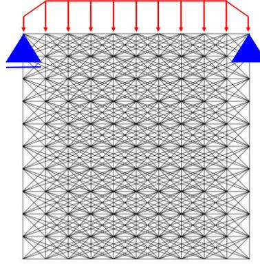
Figure 2: Example of ground-structure
