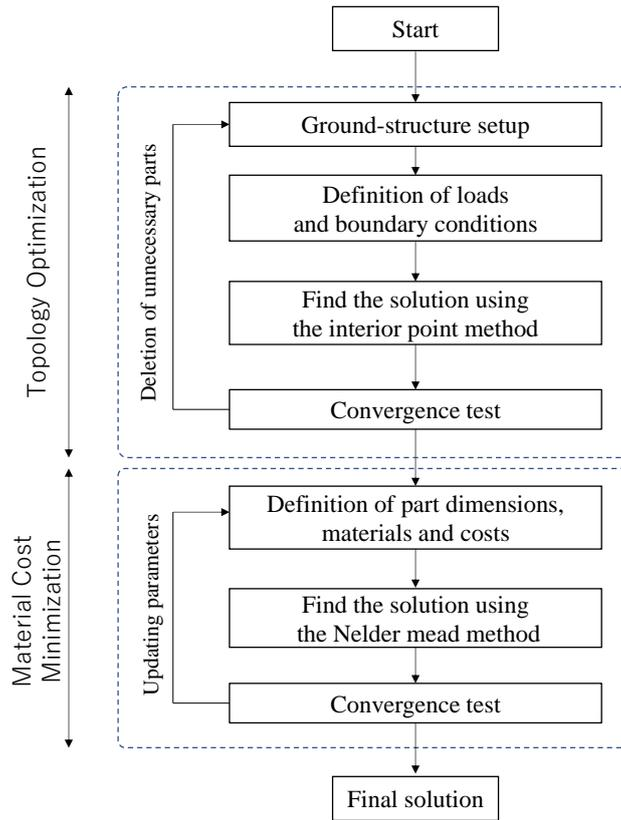
**Figure 1:** Flowchart of optimization procedure
