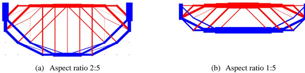
**Figure 3:** Topology optimization results (initial layout)
