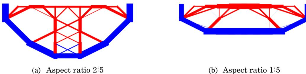
**Figure 4:** Topology optimization results (final layout)
