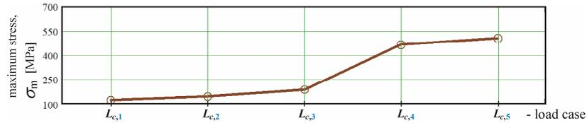
Figure 4: Graph of maximum normal stresses all over the beams of the top chord of the hybrid roof
