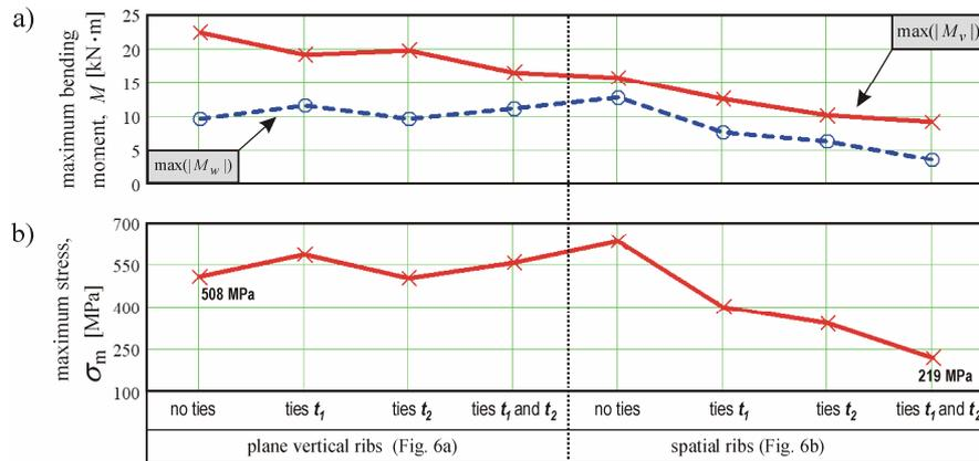
Figure 7: Analysis of the improved embodiments of the framework of the roof: a - graphs of maximum absolute bending moments in the top chord; b - graphs of maximum stresses in the top chord
