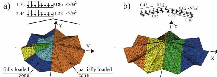
Figure 2: Non-uniform loads: a – snow load,  $L_{d,2}$ ; b - wind load,  $L_{d,3}$
