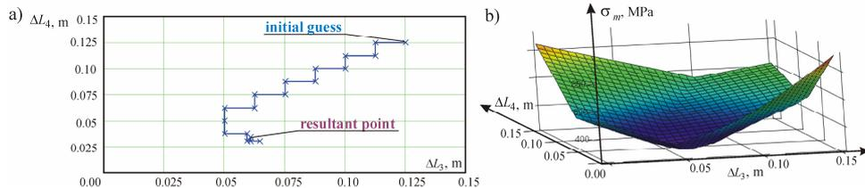
Figure 9: Obtaining the pre-tensioning values  $\Delta L_3$  and  $\Delta L_4$ . a - illustration of the optimization process; b -  $\sigma_m$ -surface given the pre-tensioning values
