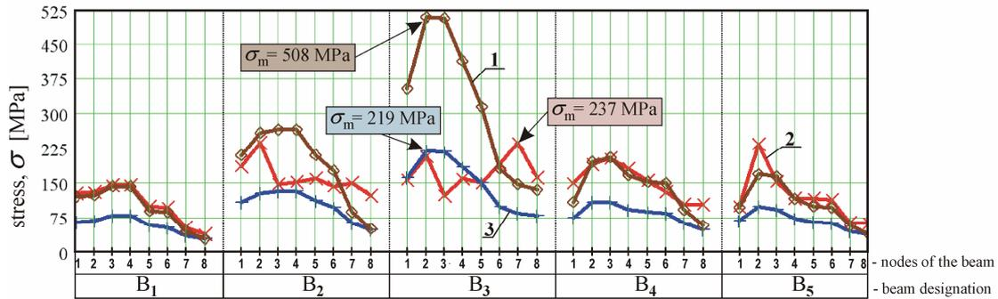
Figure 10: Diagrams of normal stresses in the top chord of the hybrid roof. 1 - reference state (no adjustment of the stresses); 2 – stress adjustment by means of simultaneous tensioning of the backstay cables; 3 – stresses in the roof's framework composed of the spatial ribs with the ties
