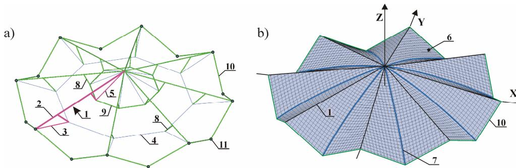
Figure 1: The hybrid roof structure. a - the framework of the roof; b - the flexible shell; 1 - the rib; 2 - the beam of the top chord; 3 - diagonal bearer cable; 4 - hoop cable; 5 - central cable; 6 - flexible polymer membrane; 7 - backstay cable; 8 - hinged strut; 9 - central ring; 10 - edge supporting beam; 11 - fixed support
