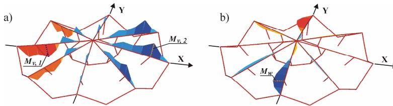
Figure 3: Diagrams of bending moments in the beams of the top chord under the load case  $L_{c,5}$  (results by EASY.2020 software<sup>10</sup>). a – the moments in the vertical plane,  $M_v$ ; b - the moments in the horizontal plane,  $M_w$
