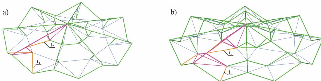
Figure 6: General structure of the improved embodiments of the framework of the roof: a – the framework of plane ribs; b – the spatial framework;  $t_1$  and  $t_2$  - supplementary flexible ties
