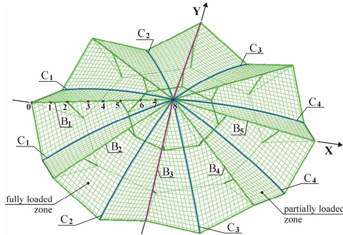
Figure 5: The top chord of the roof. Designation of the beams ( $B_1...B_5$ ), nodes ( $0...8$ ) and the backstay cables ( $C_1...C_4$ )
