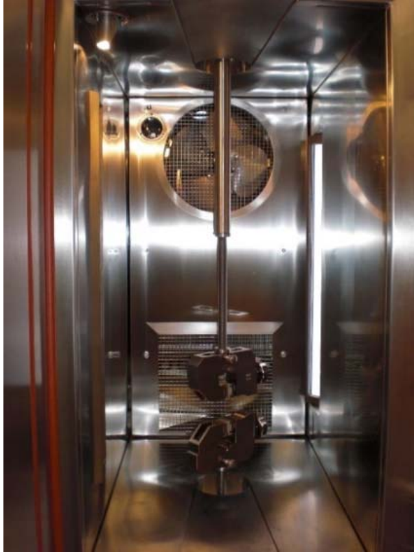
Figure 7: Uniaxial testing machine with temperature cabinet, source: seele-cover GmbH (today: se-cover GmbH) [7], cf. [2]
