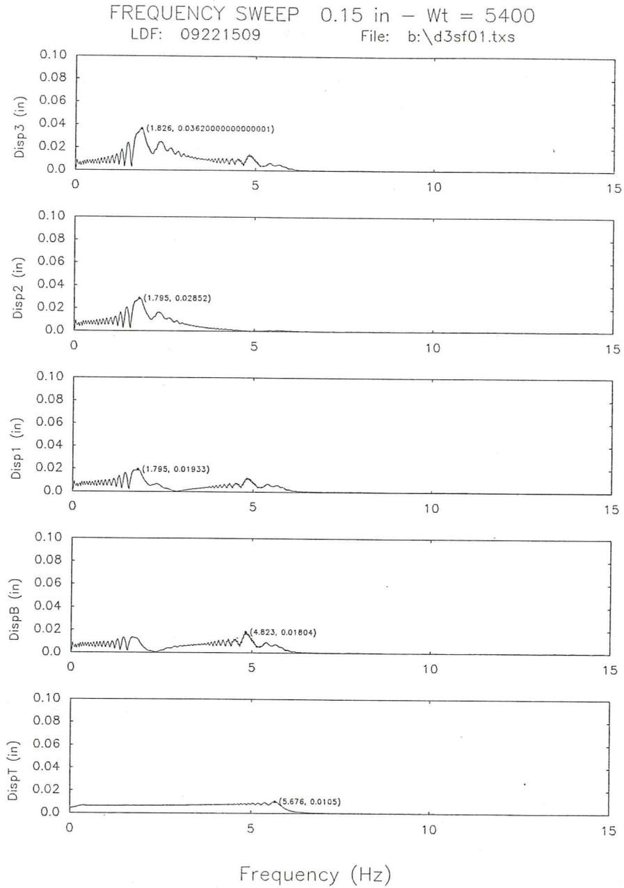
**Fig. 14d.** Fourier spectra of the displacements for the base isolated model subjected to a sweep frequency signal.
