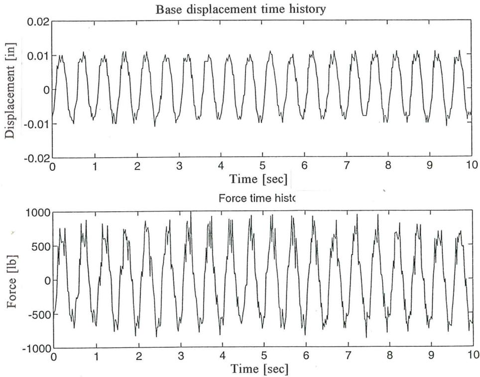
**Fig. 31f.** Base displacement time history and base shear time history for the fixed base model subjected to a sinusoidal signal ( $f=2\text{Hz}$ ). Range [500 1000].
