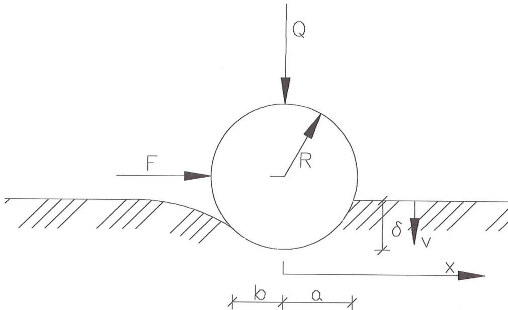
Fig. 2. Simplified model of a cylinder rolling on a rubber layer.
