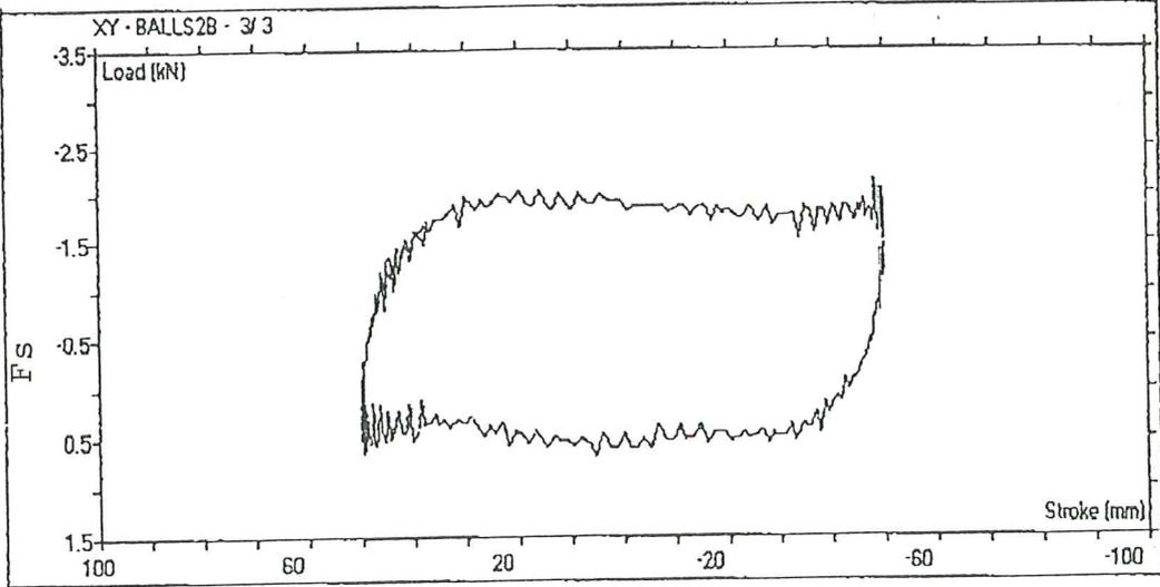
Fig. 11c. Exp.1. 4th loop of 5 loops - sinewave of 0.5 Hz ± 50mm.
