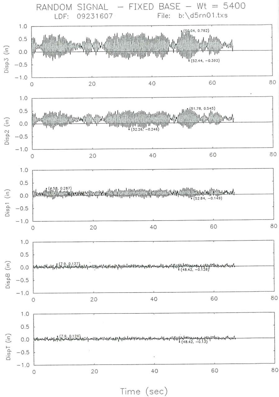
Fig. 17c. Displacement time responses for the fixed base model subjected to a random signal.
