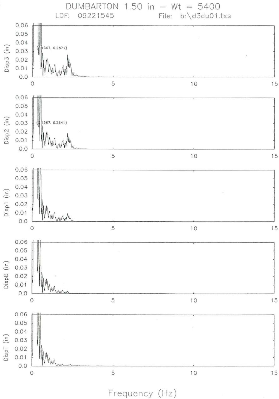
**Fig. 27d.** Fourier spectra of the displacements for the base isolated model subjected to Dumbarton signal.
