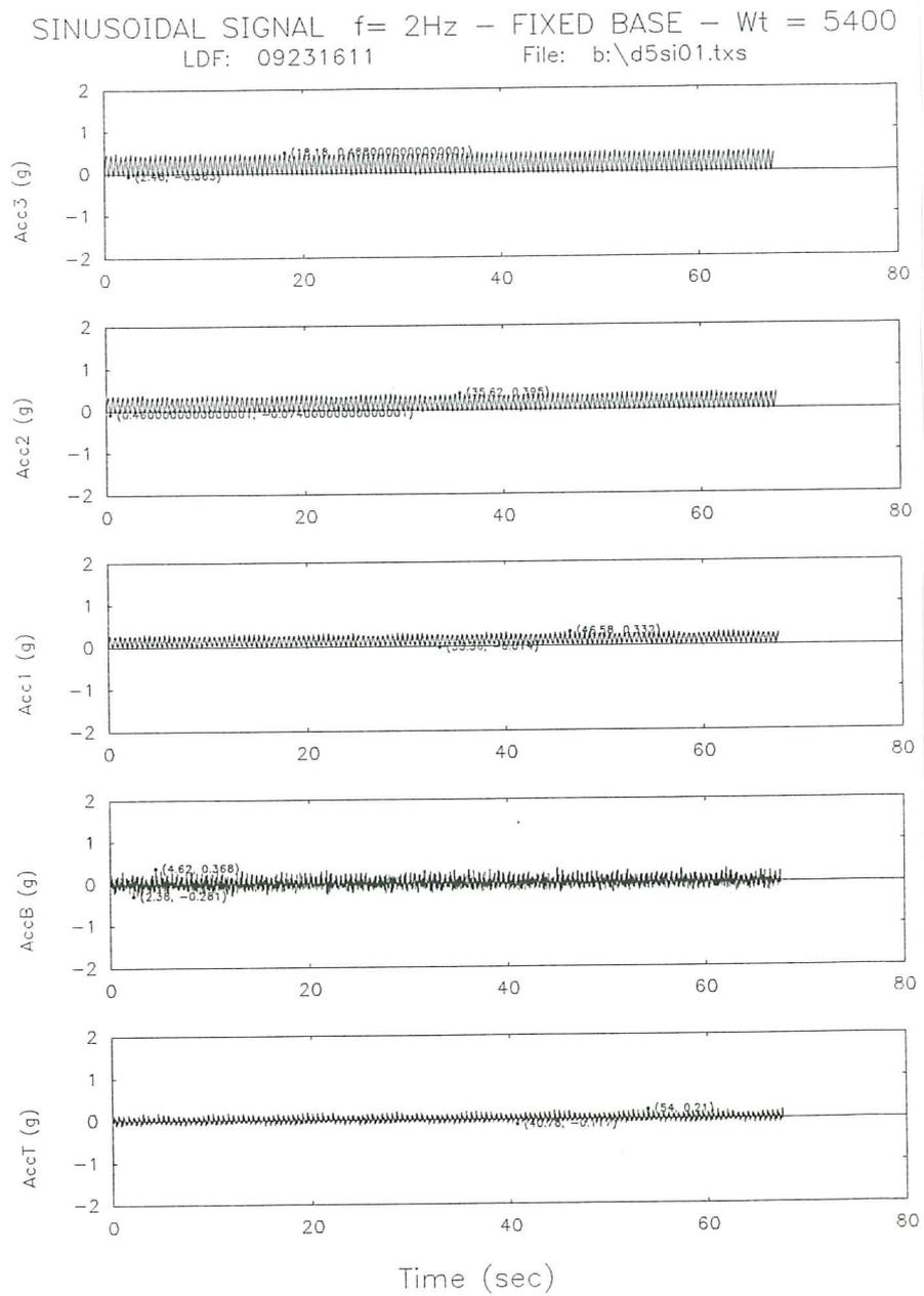
Fig. 19a. Acceleration time response for the fixed base model subjected to a sinusoidal signal ( $f=2\text{Hz}$ ).
