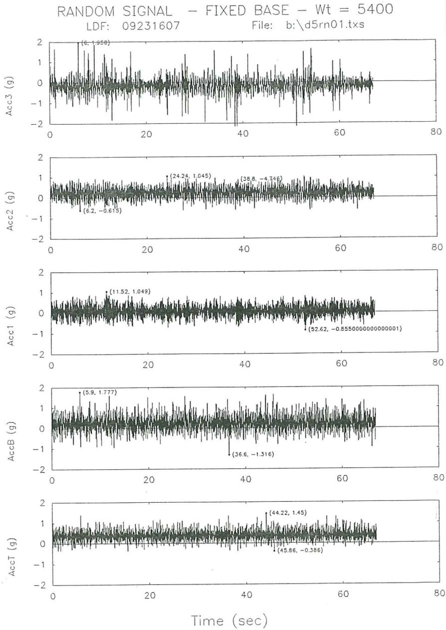
Fig. 17a. Acceleration time response for the fixed base model subjected to a random signal.
