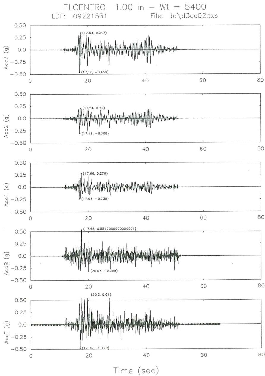
Fig. 23a. Acceleration time response for the base isolated model subjected to El Centro signal.
