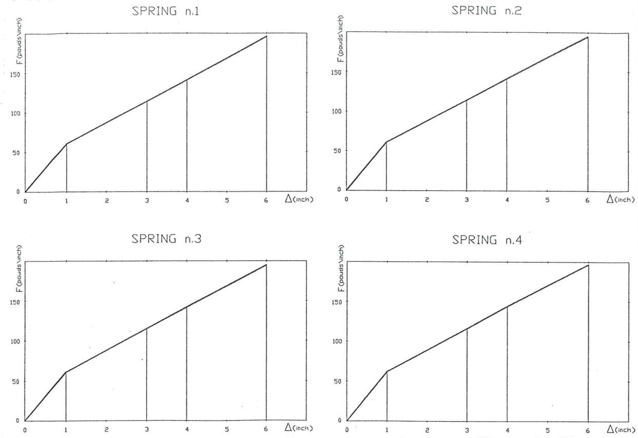
Fig. 8. Stiffnesses of the springs. Experimental F-δ diagrams.
