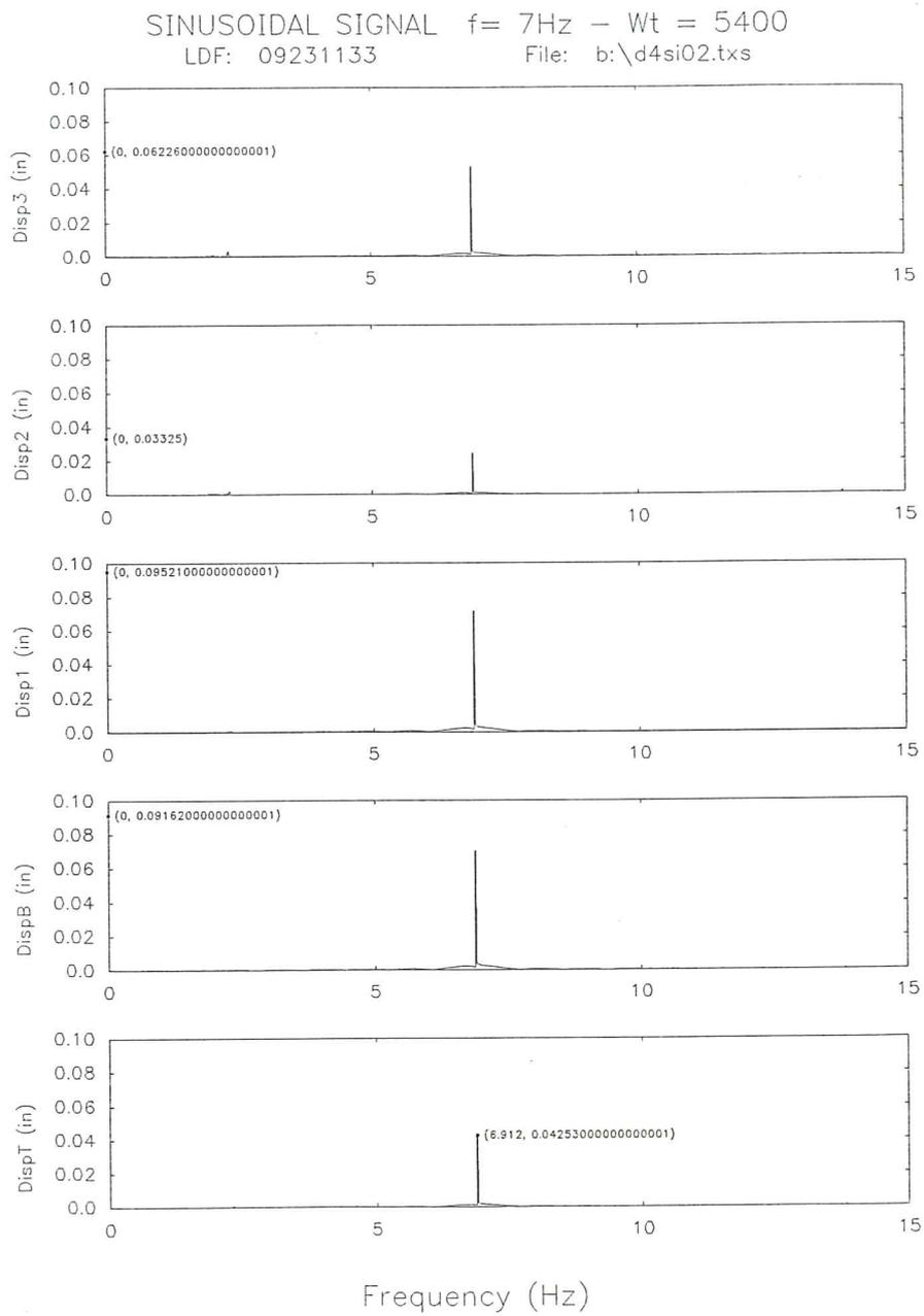
Fig. 20d. Fourier spectra of the displacements for the base isolated model subjected to a sinusoidal signal ( $f=7\text{Hz}$ ).
