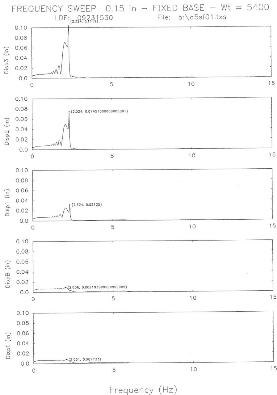
Fig. 15d. Fourier spectra of the displacements for the fixed base model subjected to a sweep frequency signal.
