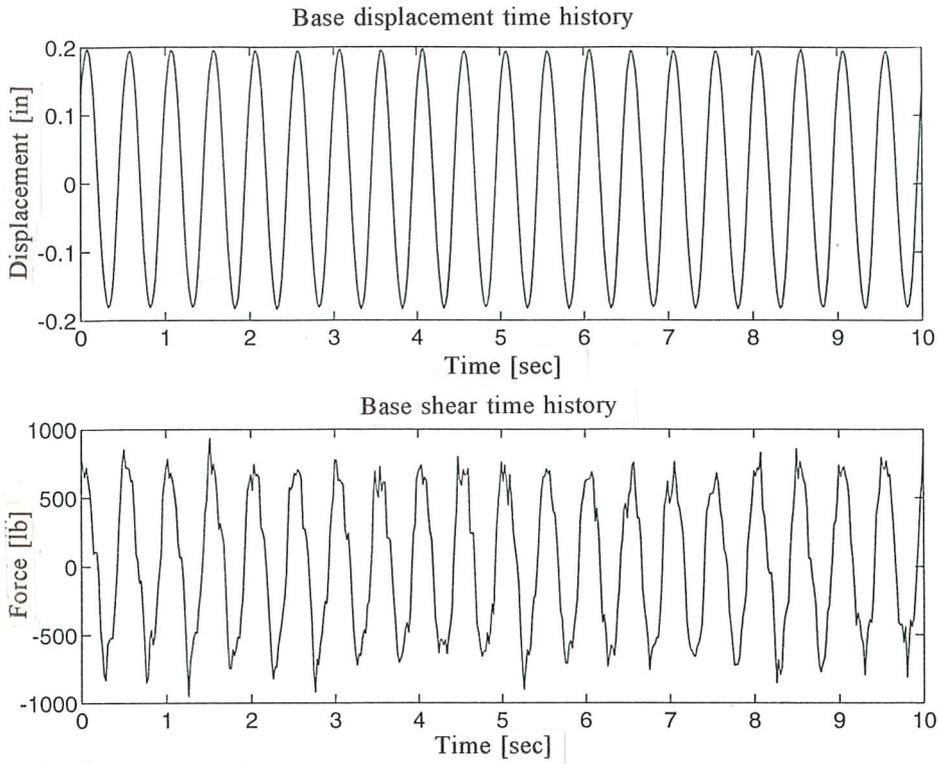
**Fig. 31e.** Base displacement time history and base shear time history for the base isolated model subjected to a sinusoidal signal ( $f=2\text{Hz}$ ). Range [500 1000].
