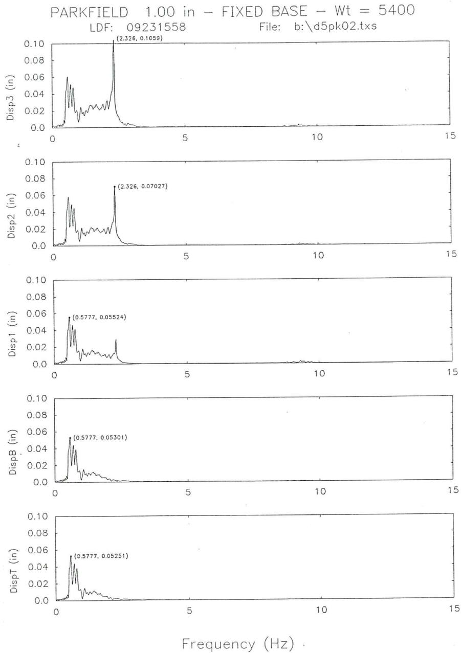
**Fig. 26d.** Fourier spectra of the displacements for the fixed base model subjected to Parkfield signal.
