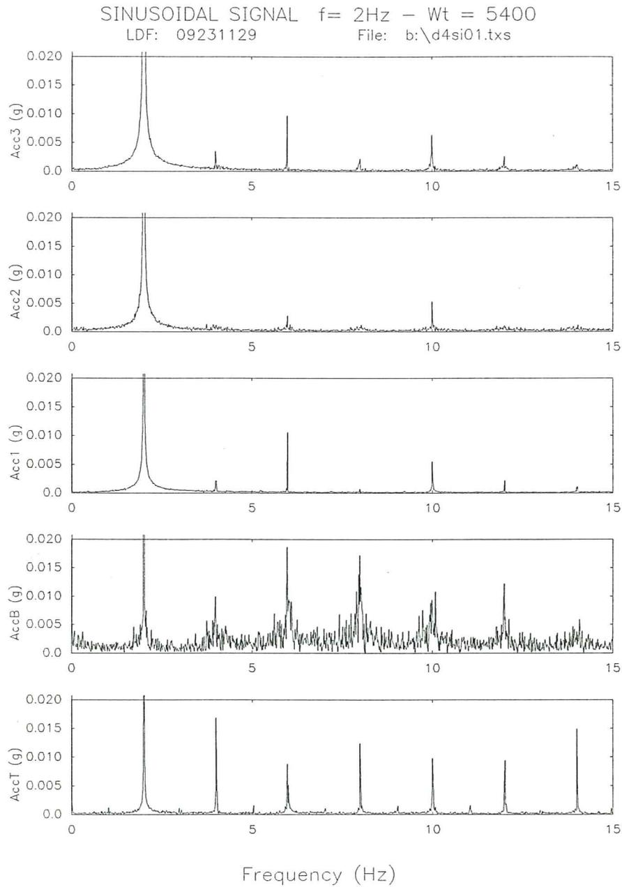
**Fig. 18b.** Fourier spectra of the accelerations for the base isolated model subjected to a sinusoidal signal ( $f=2\text{Hz}$ ).
