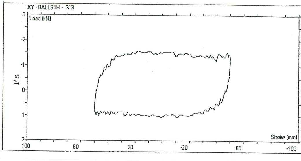
Fig. 10c. Exp.1. 4th loop of 5 loops - sinewave of 0.1 Hz  $\pm$  50mm.
