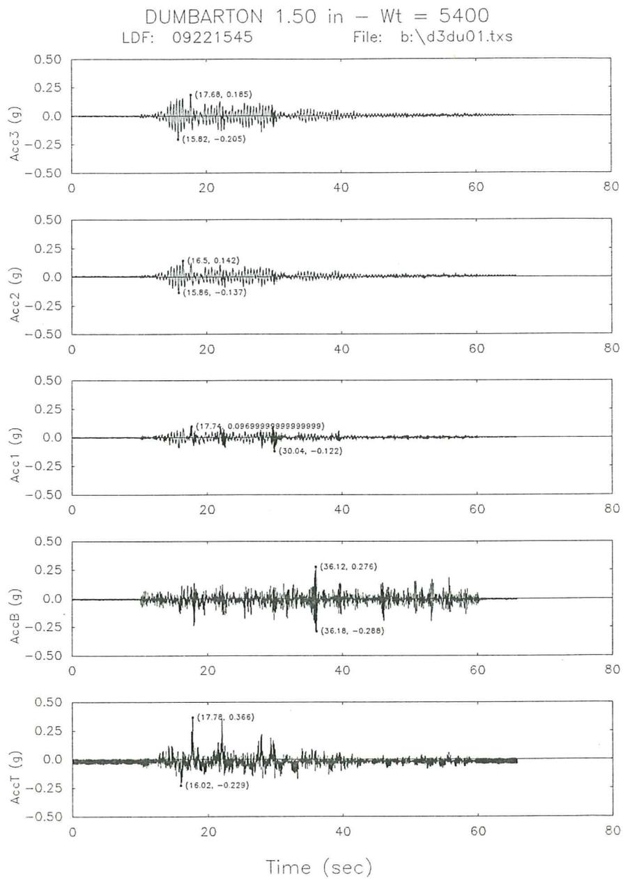
Fig. 27a. Acceleration time response for the base isolated model subjected to Dumbarton signal.
