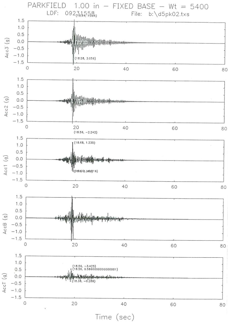
Fig. 26a. Acceleration time response for the fixed base model subjected to Parkfield signal.
