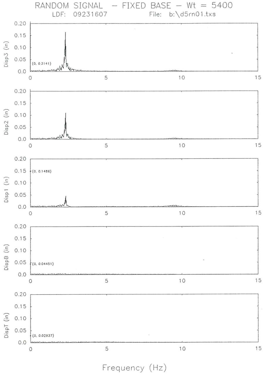
Fig. 17d. Fourier spectra of the displacements for the fixed base model subjected to a random signal.
