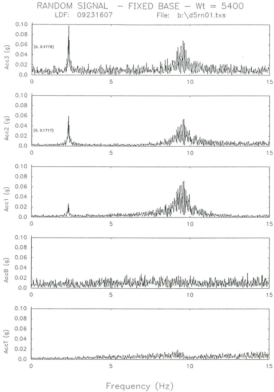
**Fig. 17b.** Fourier spectra of the accelerations for the fixed base model subjected to a random signal.
