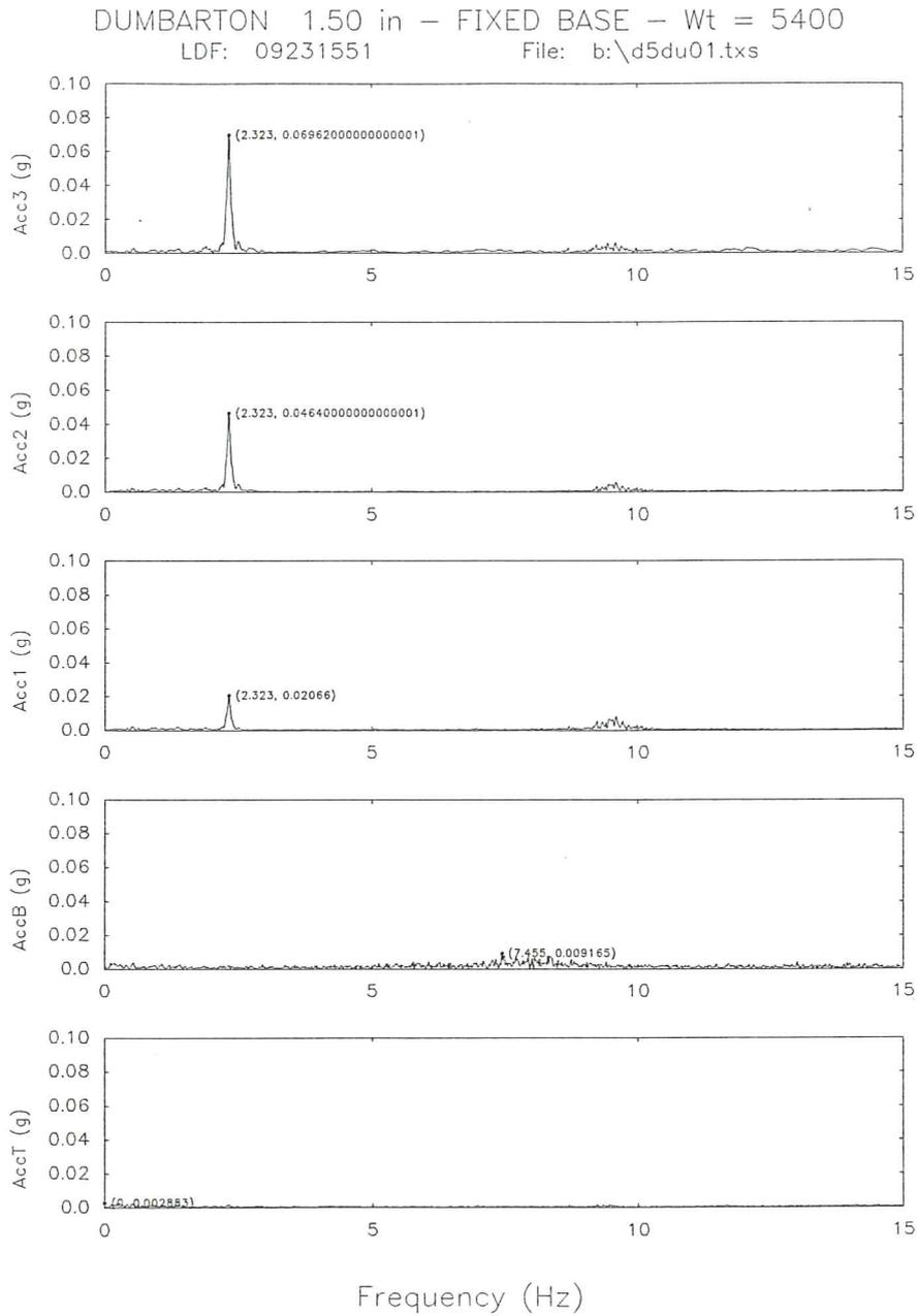
**Fig. 28b.** Fourier spectra of the accelerations for the fixed base model subjected to Dumbarton signal.
