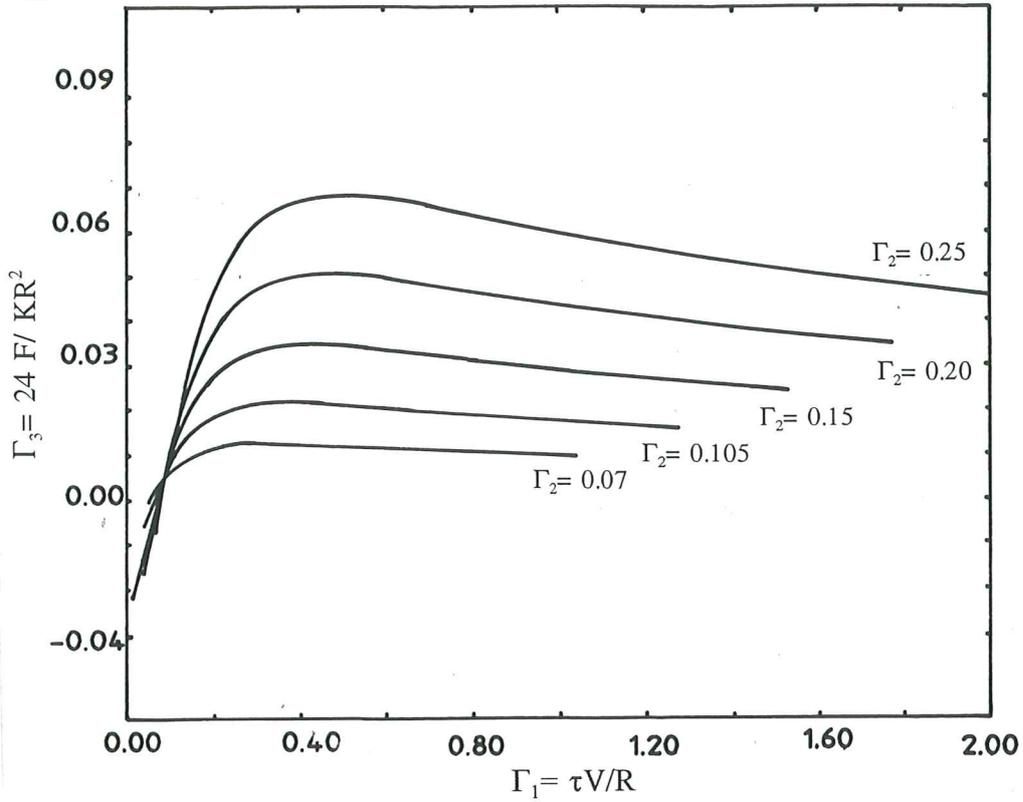
Fig. 3b. Dimensionless velocity V-Force F diagrams for different values of the vertical load Q.
