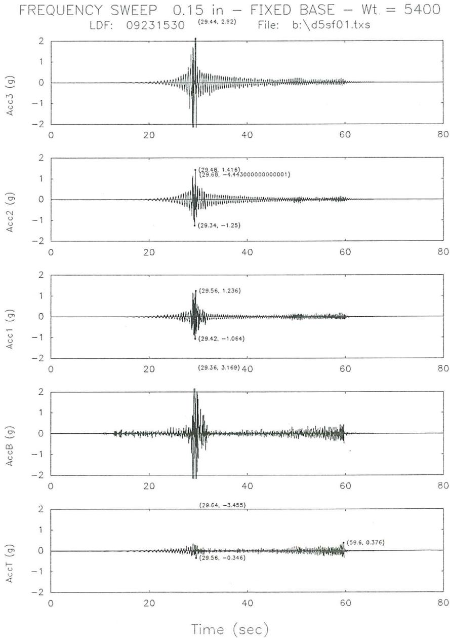
Fig. 15a. Acceleration time response for the fixed base model subjected to a sweep frequency signal.
