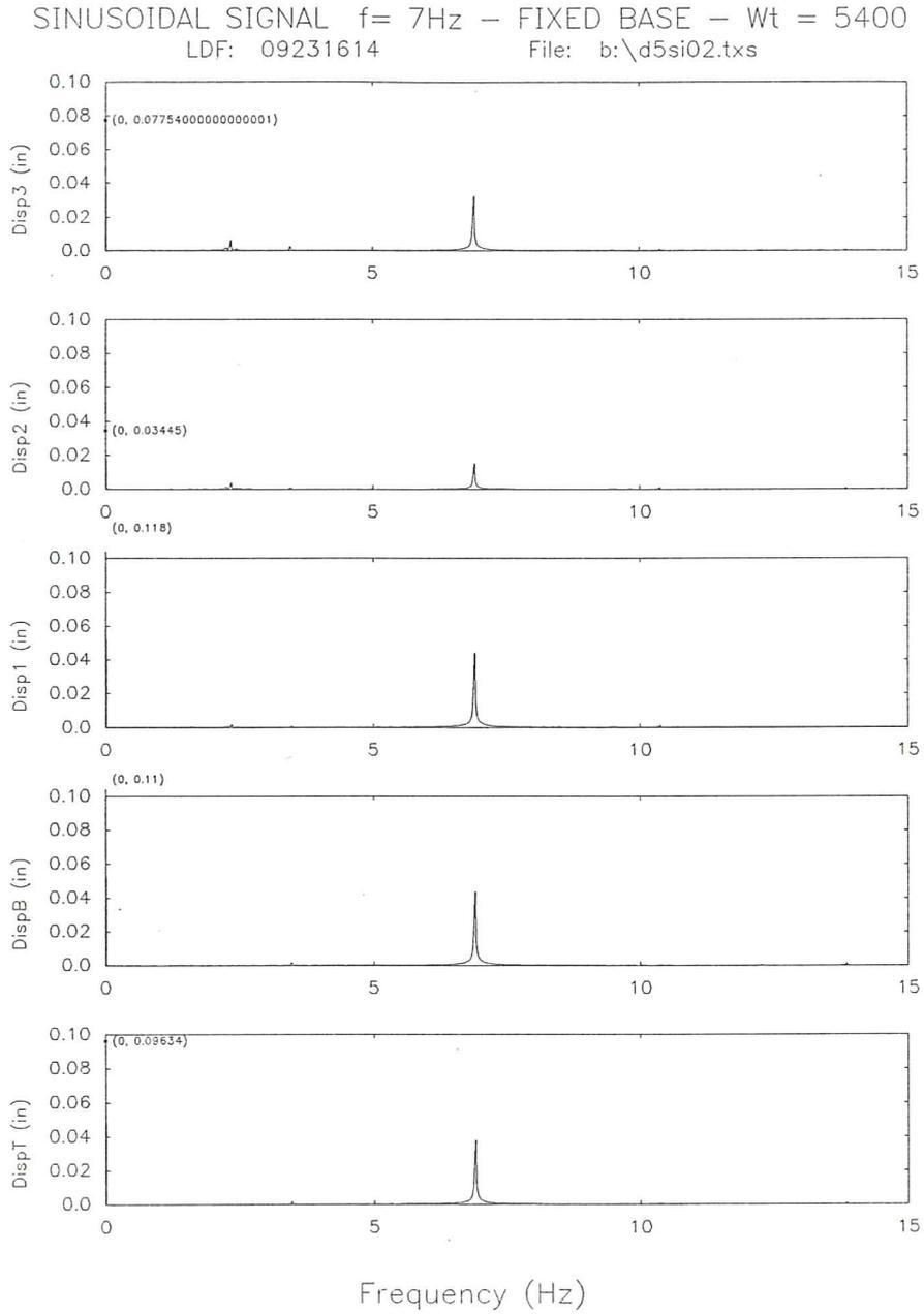
**Fig. 21d.** Fourier spectra of the displacements for the fixed base model subjected to a sinusoidal signal ( $f=7\text{Hz}$ ).
