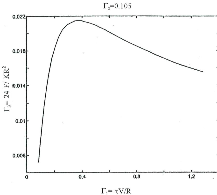
Fig. 3a. Dimensionless velocity  $V$ -Force  $F$  diagram for a fixed vertical load  $Q=50$  pounds.
