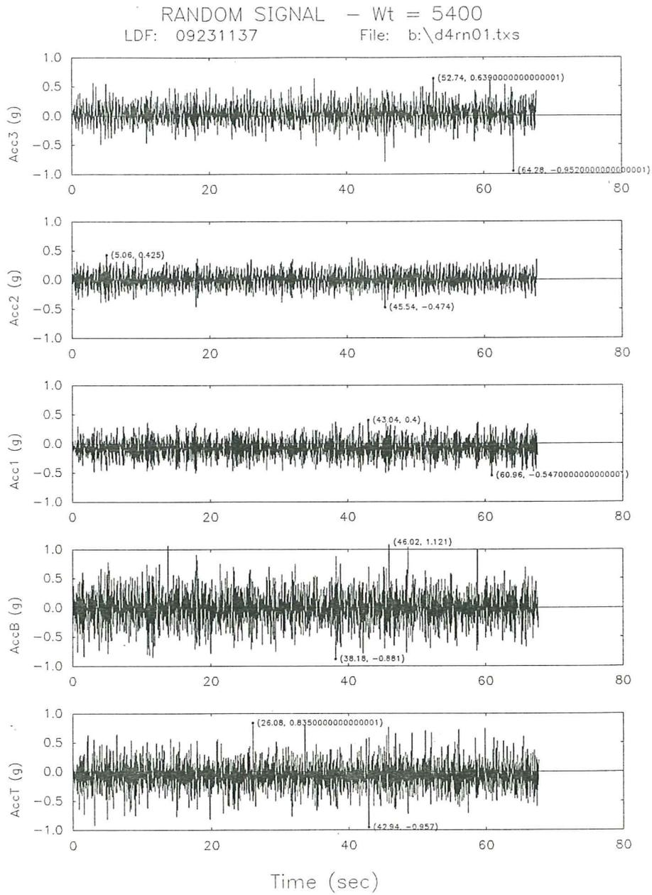
Fig. 16a. Acceleration time response for the base isolated model subjected to a random signal.
