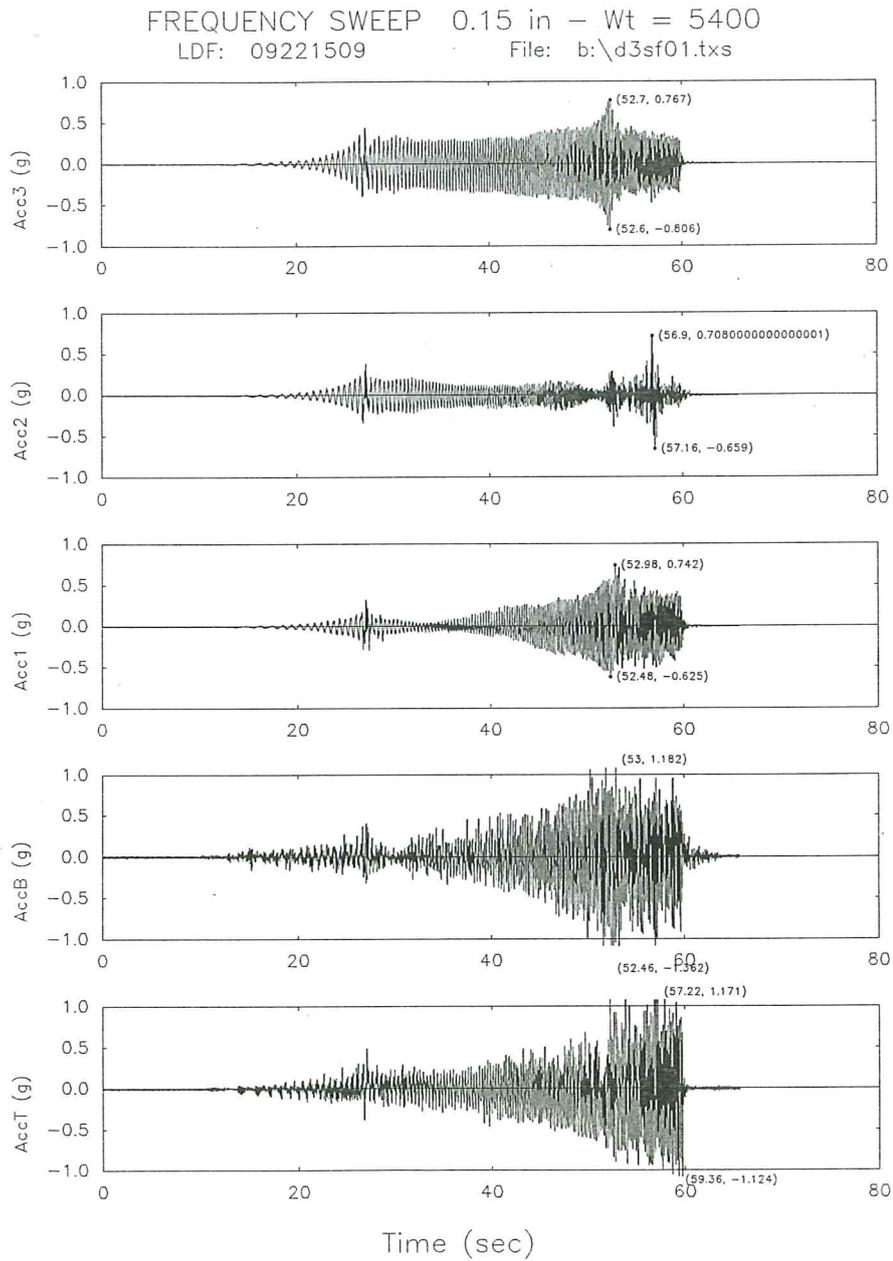
Fig. 14a. Acceleration time response for the base isolated model subjected to a sweep frequency signal.
