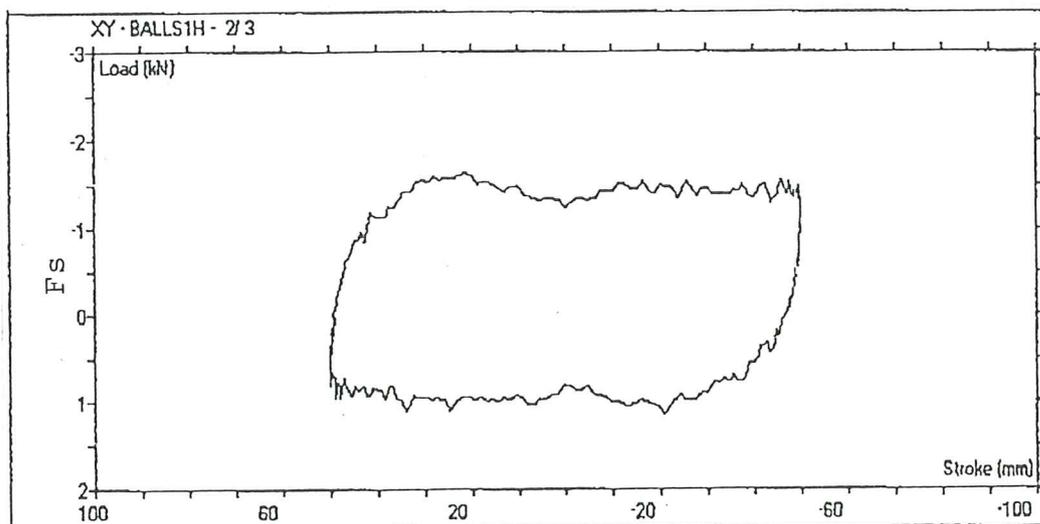
Fig. 10b. Exp.1. 2nd loop of 5 loops - sinewave of 0.1 Hz  $\pm$  50mm.
