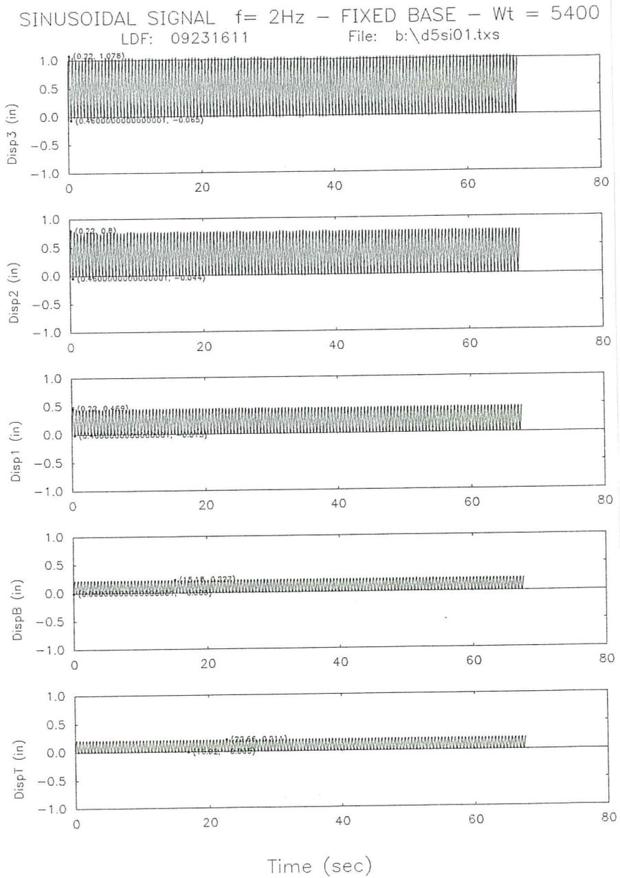
Fig. 19c. Displacement time responses for the fixed base model subjected to a sinusoidal signal ( $f=2\text{Hz}$ ).
