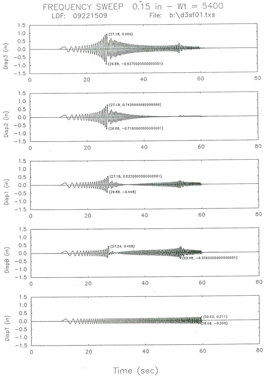
Fig. 14c. Displacement time responses for the base isolated model subjected to a sweep frequency signal.
