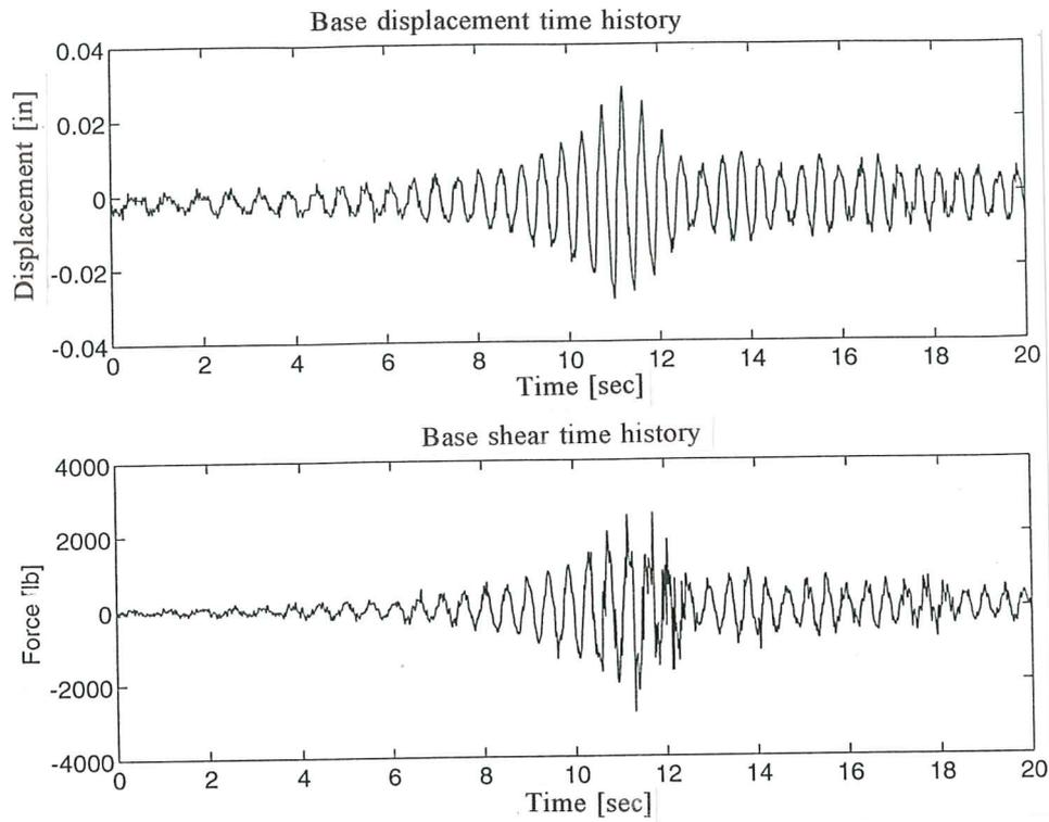
**Fig. 31c.** Base displacement time history and base shear time history for the fixed base model subjected to a sweep frequency signal. Range [1000 2000].
