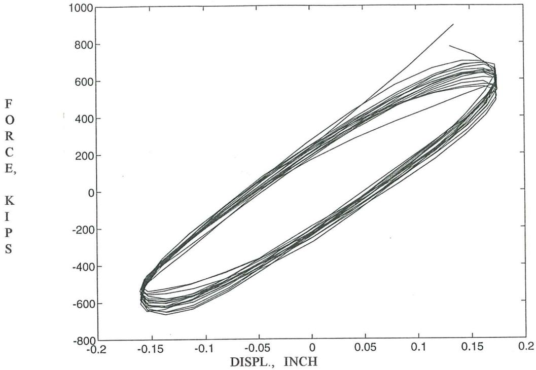
SINUSOIDAL SIGNAL  $f=2\text{Hz}$  - Fixed Base -  $W_t=5360\text{ lb}$
