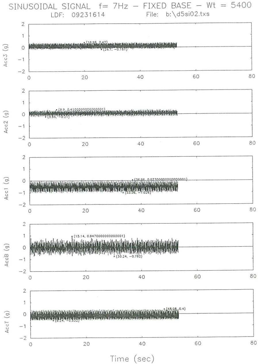
Fig. 21a. Acceleration time response for the fixed base model subjected to a sinusoidal signal ( $f=7\text{Hz}$ ).
