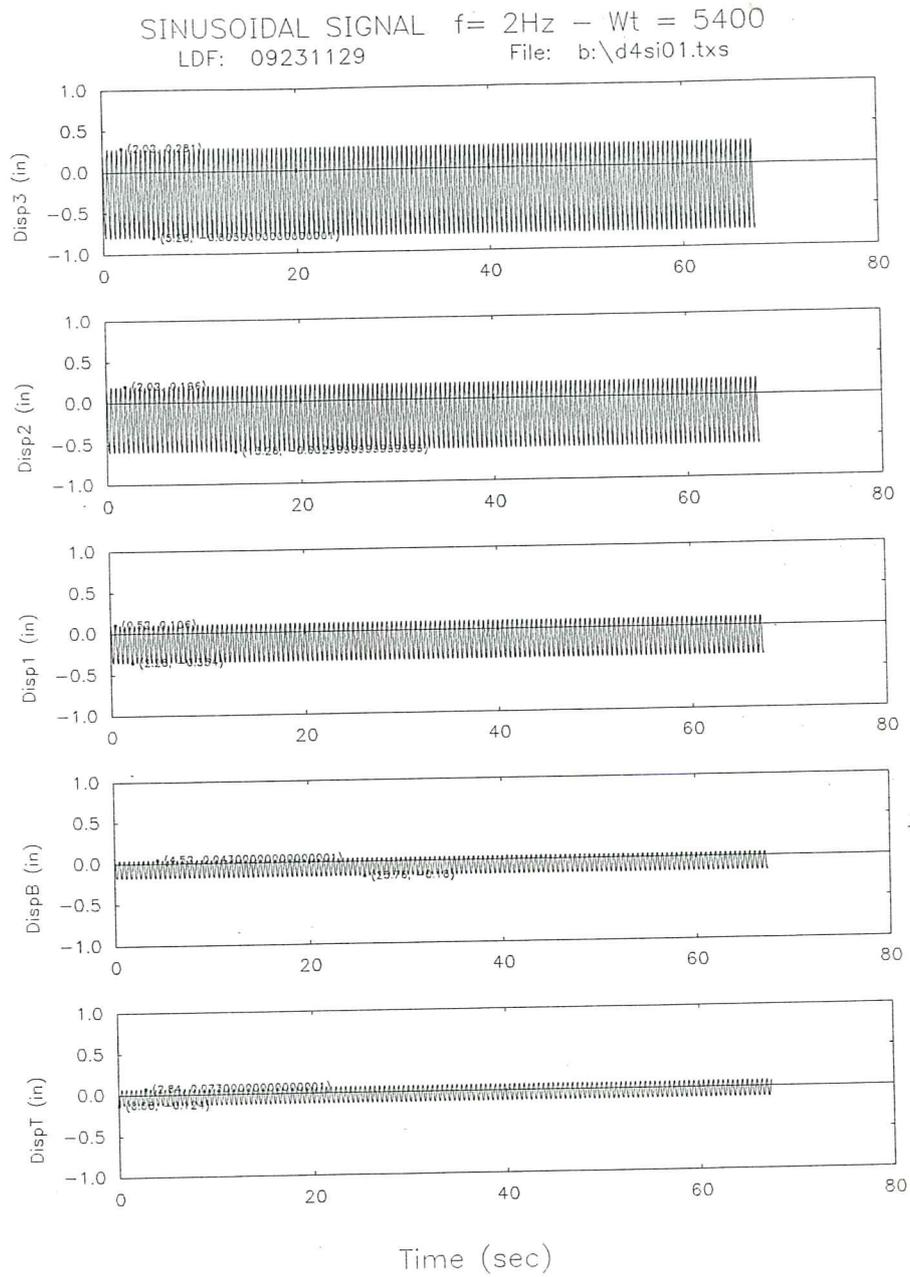
Fig. 18c. Displacement time response for the base isolated model subjected to a sinusoidal signal ( $f=2\text{Hz}$ ).
