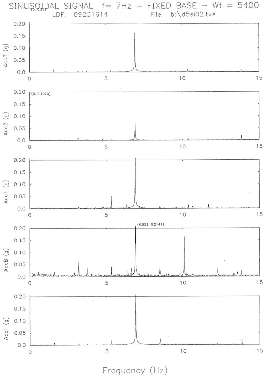
Fig. 21b. Fourier spectra of the accelerations for the fixed base model subjected to a sinusoidal signal ( $f=7\text{Hz}$ ).
