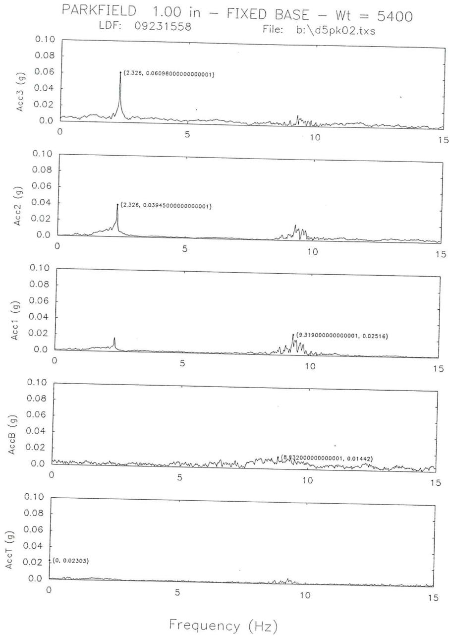
**Fig. 26b.** Fourier spectra of the accelerations for the fixed base model subjected to Parkfield signal.
