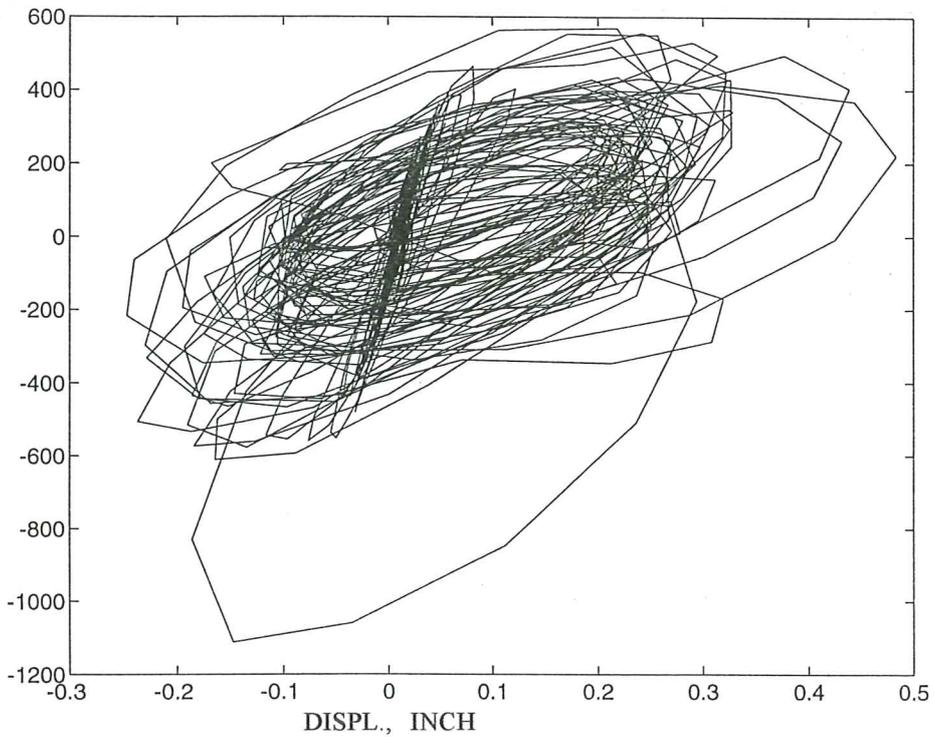
Fig. 30c. Base shear hysteresis loops for the base isolated model subjected to a sweep frequency signal.
