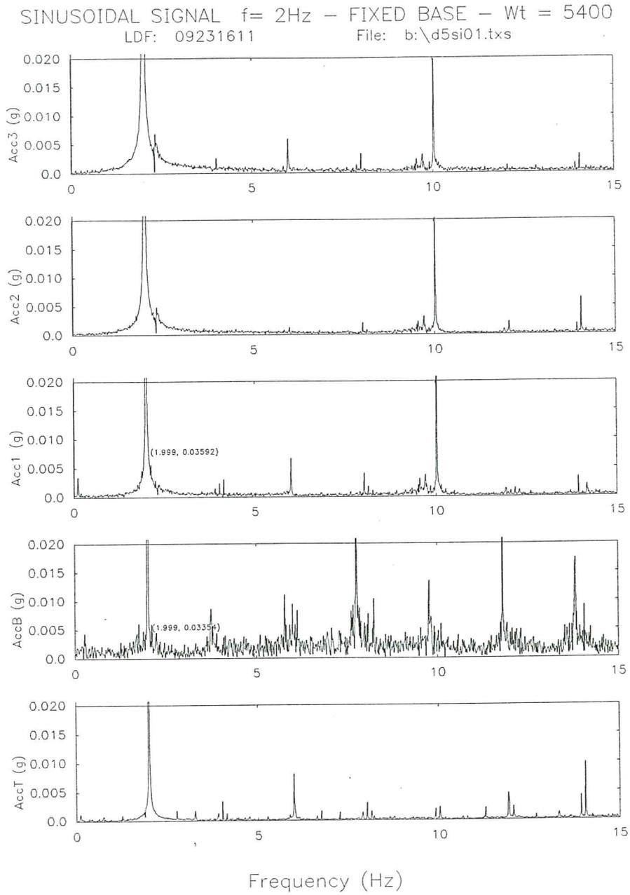
**Fig. 19b.** Fourier spectra of the accelerations for the fixed base model subjected to a sinusoidal signal ( $f=2\text{Hz}$ ).
