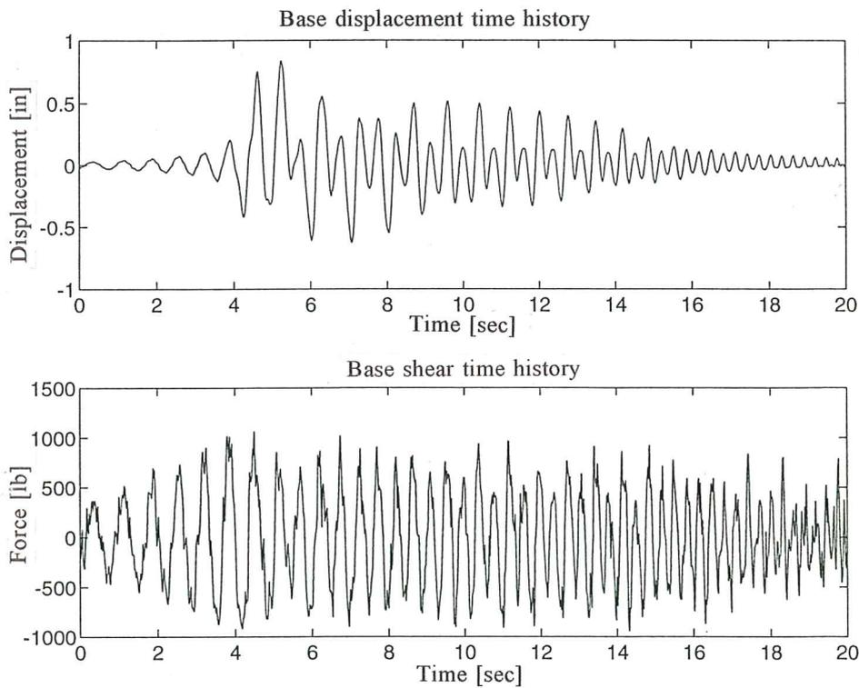
**Fig. 31b.** Base displacement time history and base shear time history for the base isolated model subjected to a sweep frequency signal. Range [2000 3000].
