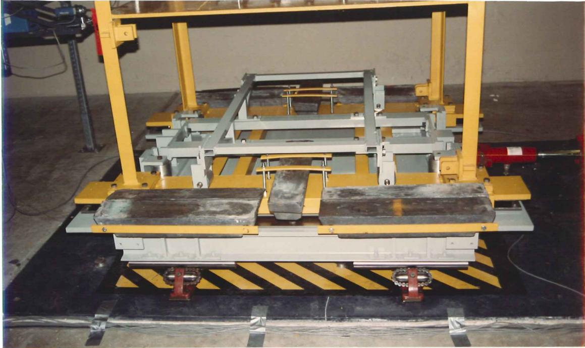
**Photo 5.** The isolated base of the model frame.
