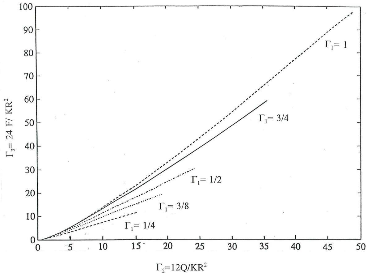
Fig. 5. Dimensionless vertical load Q-Force F diagram for different values of the velocity  $V$ .
