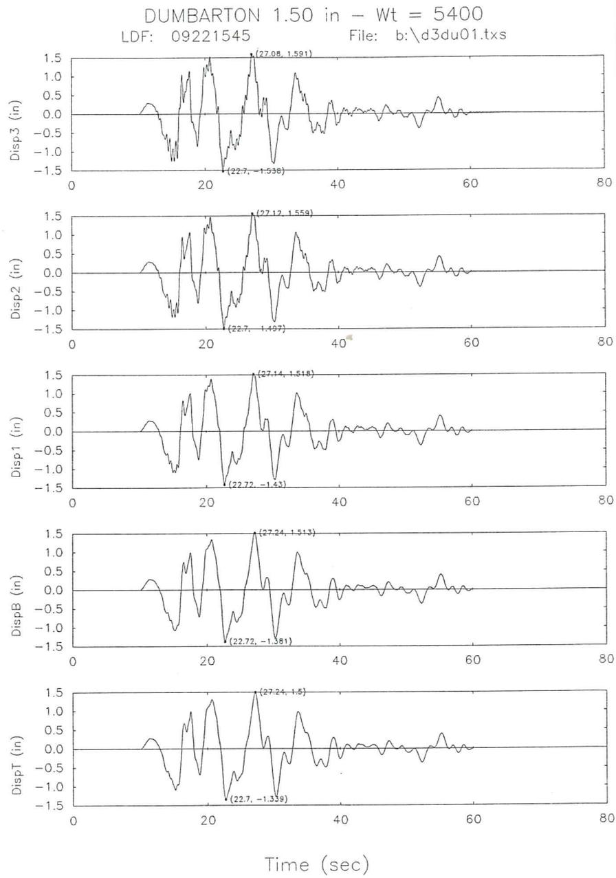
Fig. 27c. Displacement time responses for the base isolated model subjected to Dumbarton signal.
