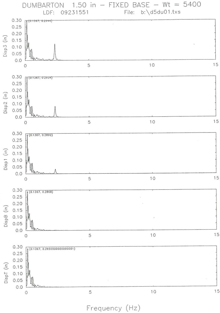
**Fig. 28d.** Fourier spectra of the displacements for the fixed base model subjected to Dumbarton signal.
