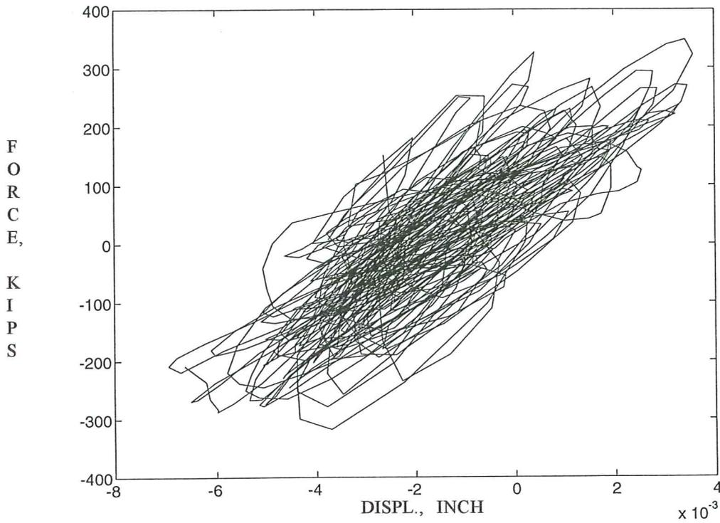
Fig. 30d. Base shear hysteresis loops for the fixed base model subjected to a sweep frequency signal.
