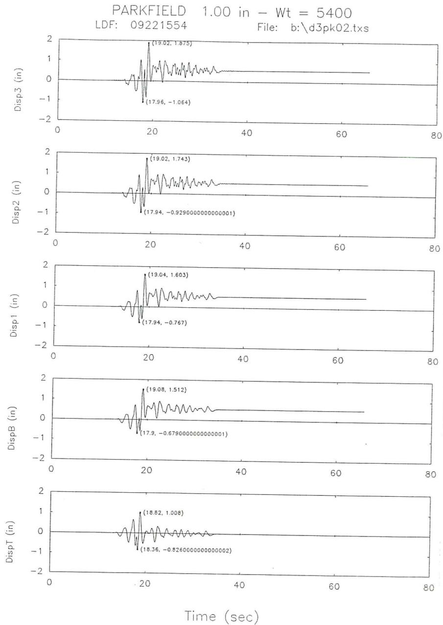
**Fig. 25c.** Displacement time responses for the base isolated model subjected to Parkfield signal.
