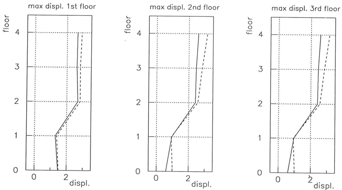
**Fig. 29c.** Deflected shape at maximum story displacements for El Centro signal and Dumbarton signal.
