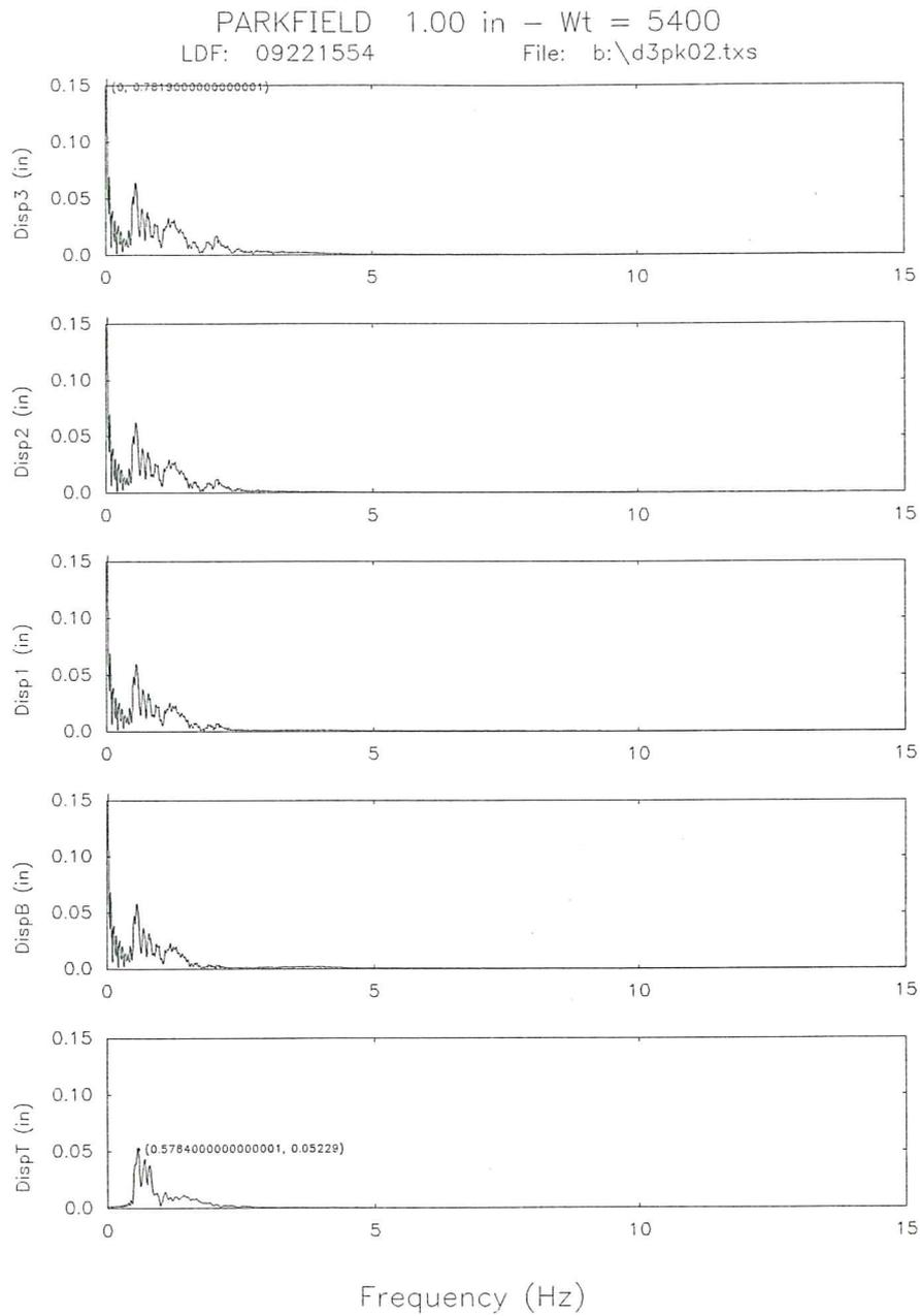
Fig. 25d. Fourier spectra of the displacements for the base isolated model subjected to Parkfield signal.
