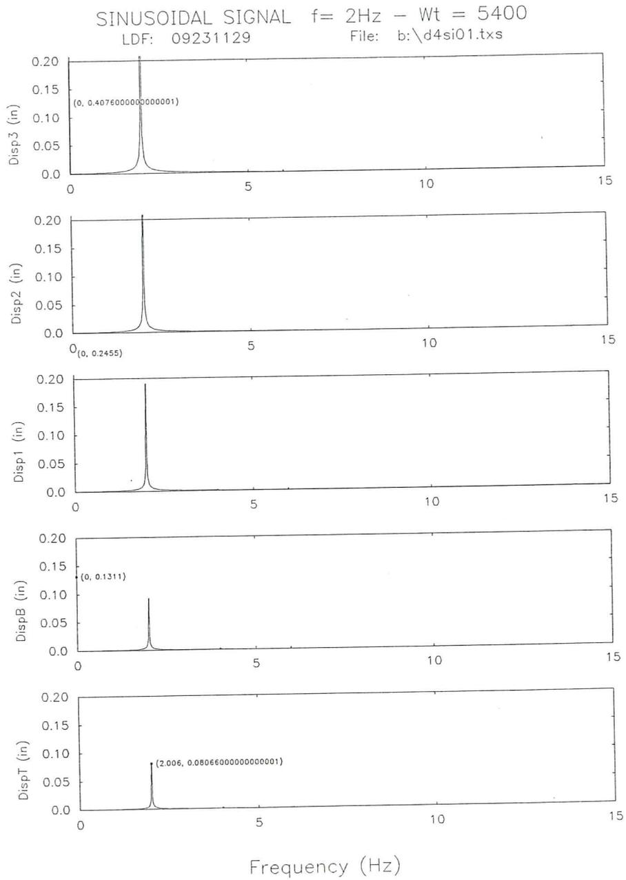
**Fig. 18d.** Fourier spectra of the displacements for the base isolated model subjected to a sinusoidal signal ( $f=2\text{Hz}$ ).
