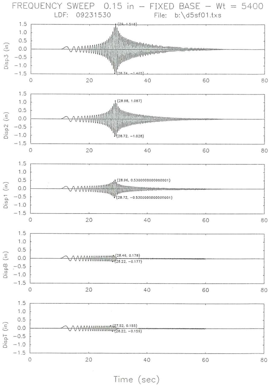
Fig. 15c. Displacement time responses for the fixed base model subjected to a sweep frequency signal.
