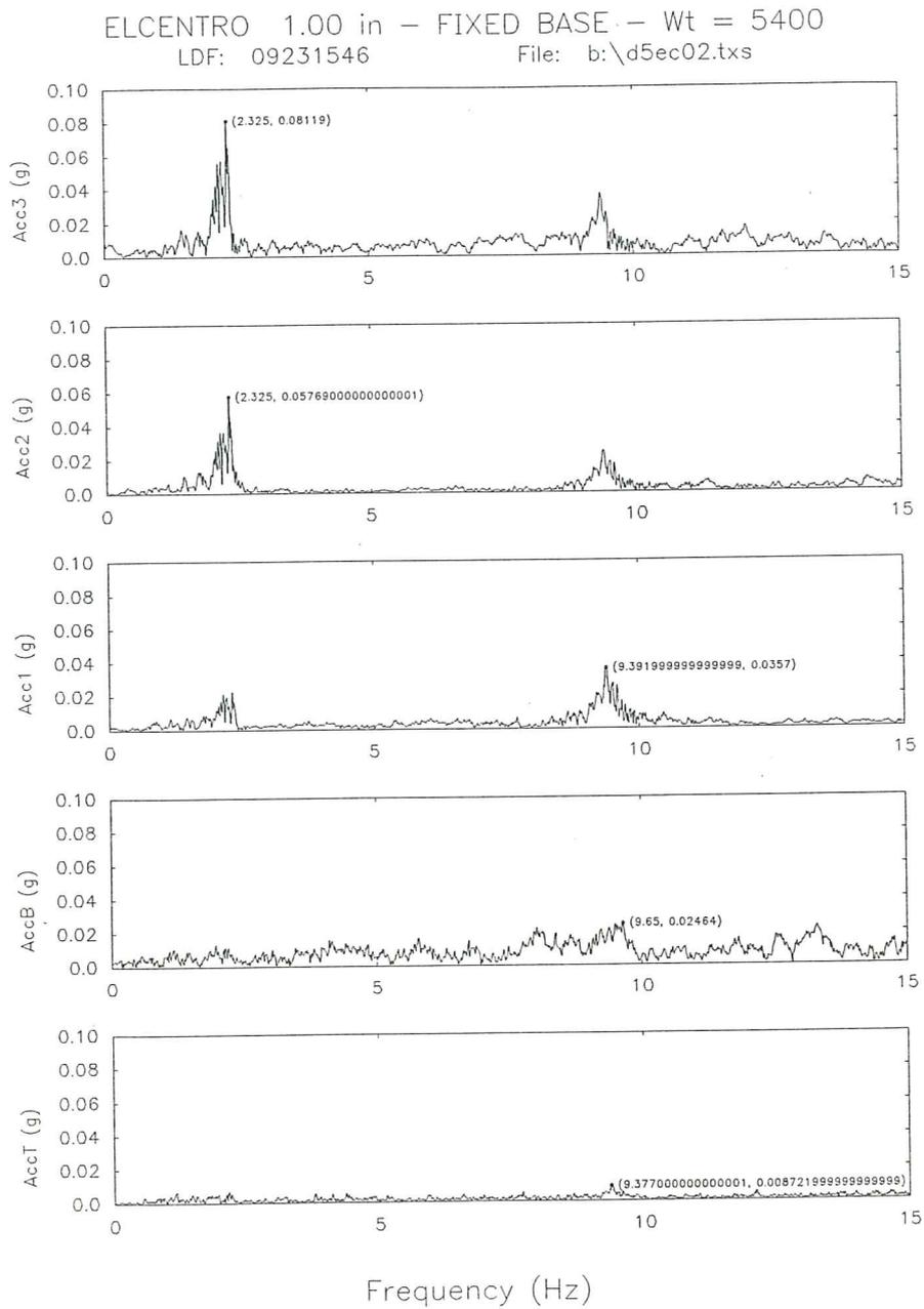
**Fig. 24b.** Fourier spectra of the accelerations for the fixed base model subjected to El Centro signal.
