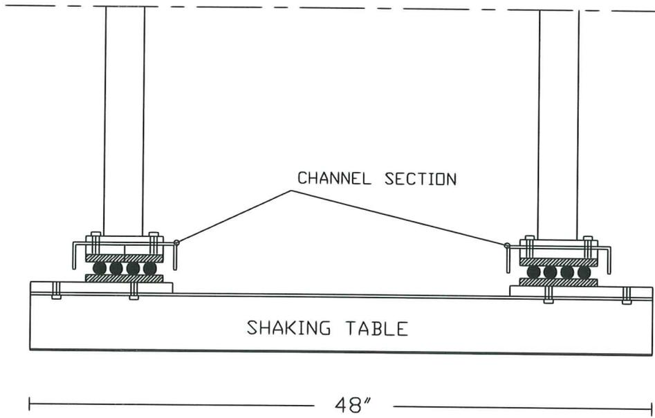
Fig. 1a. Longitudinal section of the isolation system.
