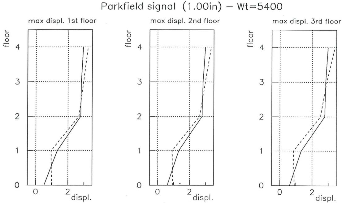
**Fig. 29d.** Deflected shape at maximum story displacements for Parkfield signal.
