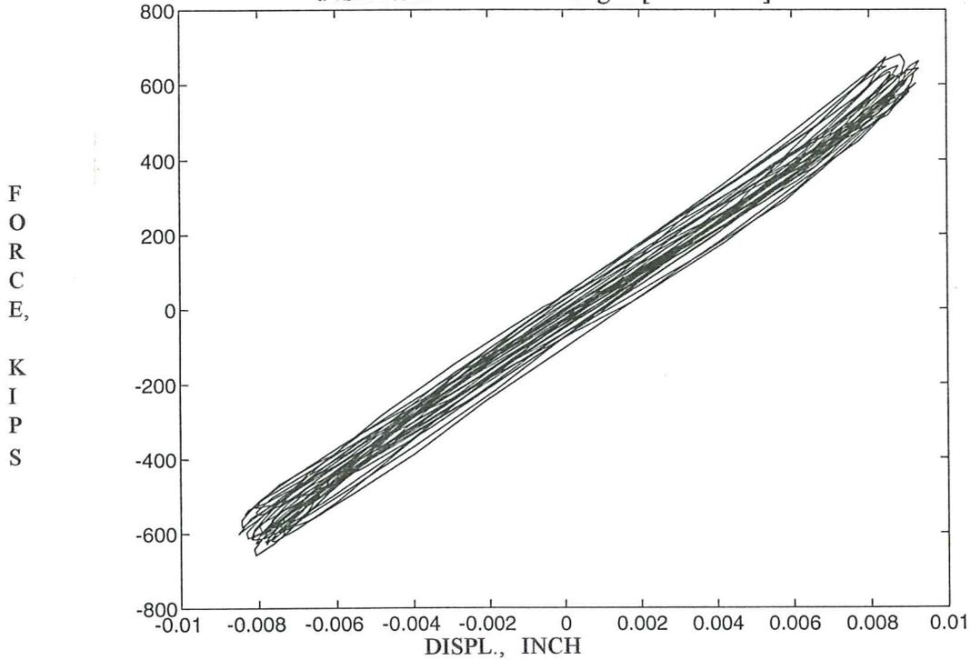
Fig. 30b. Base shear hysteresis loops for the base isolated and fixed base model subjected to a sinusoidal signal.
