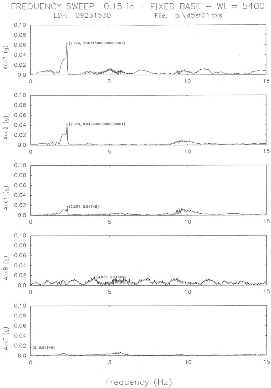
Fig. 15b. Fourier spectra of the accelerations for the fixed base model subjected to a sweep frequency signal.
