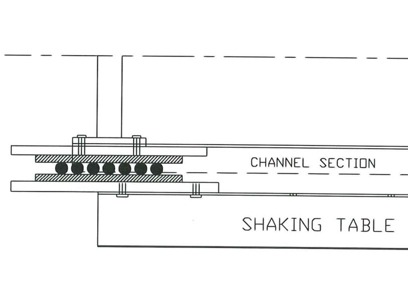
Fig. 1b. Transversal section of the isolation system.
