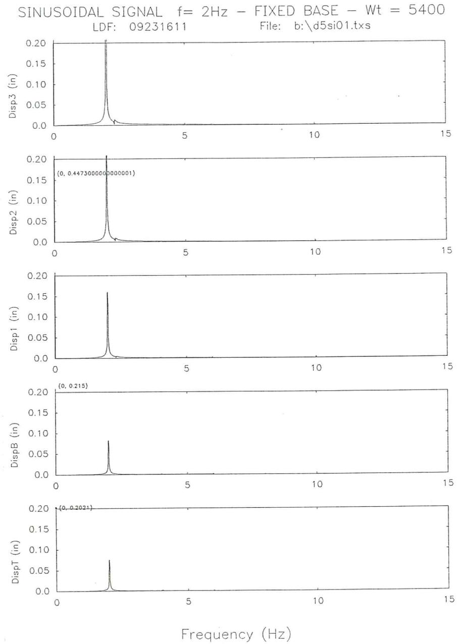
Fig. 19d. Fourier spectra of the displacements for the fixed base model subjected to a sinusoidal signal ( $f=2\text{Hz}$ ).
