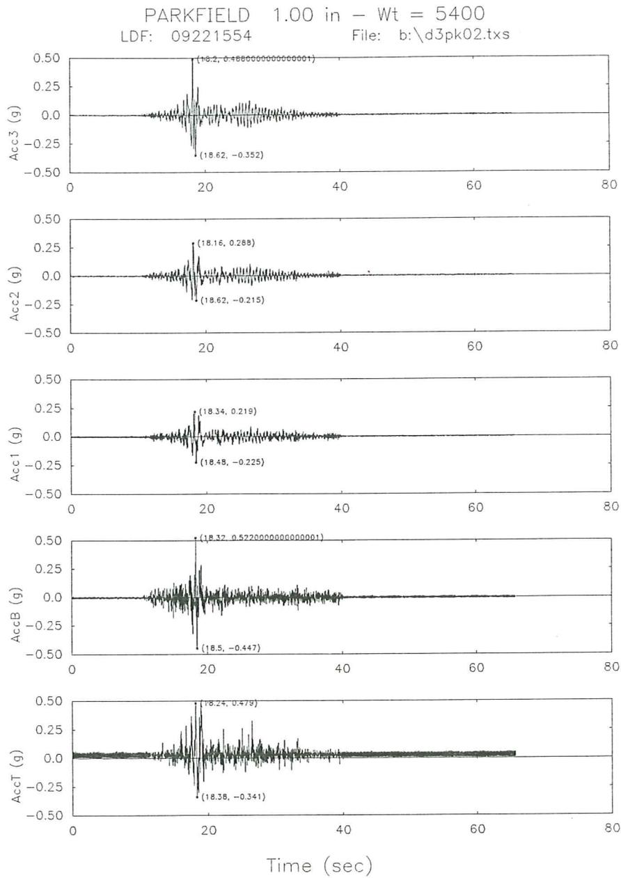
Fig. 25a. Acceleration time response for the base isolated model subjected to Parkfield signal.
