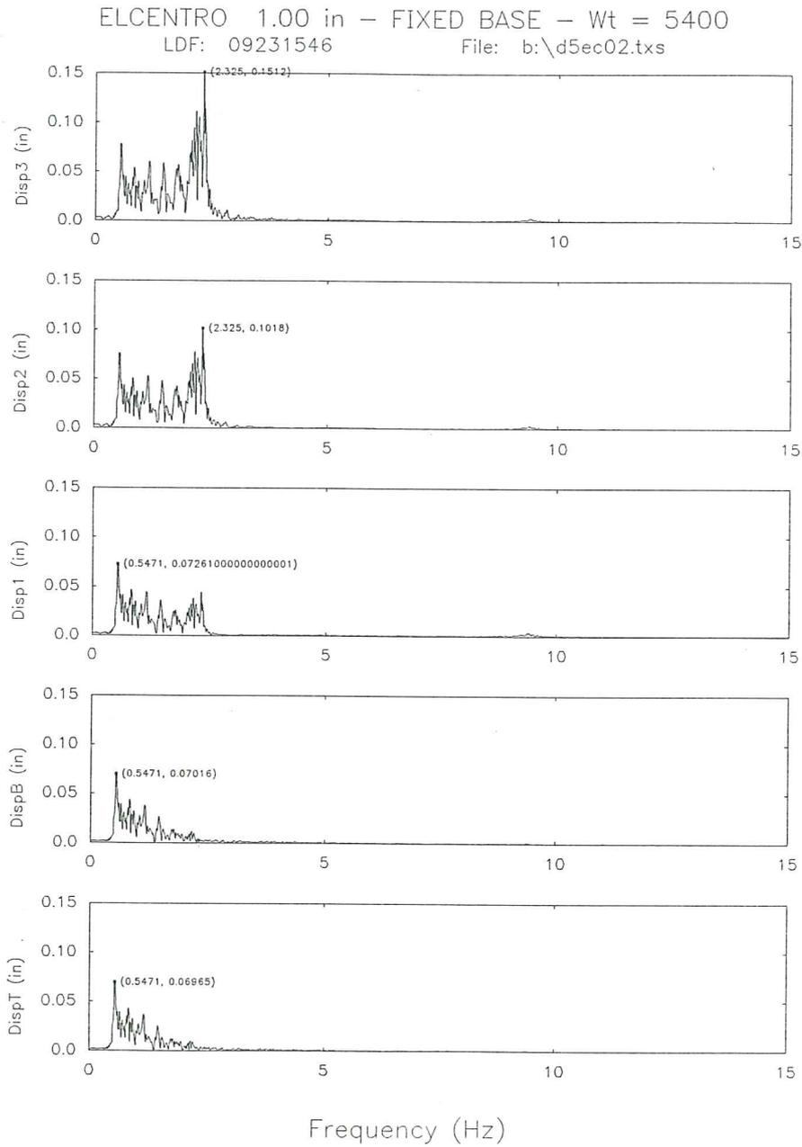
**Fig. 24d.** Fourier spectra of the displacements for the fixed base model subjected to El Centro signal.
