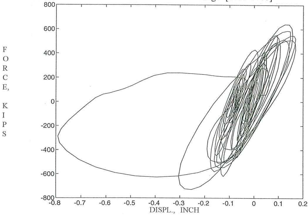
Fig. 30a. Base shear hysteresis loops for the base isolated model subjected to El Centro signal.
