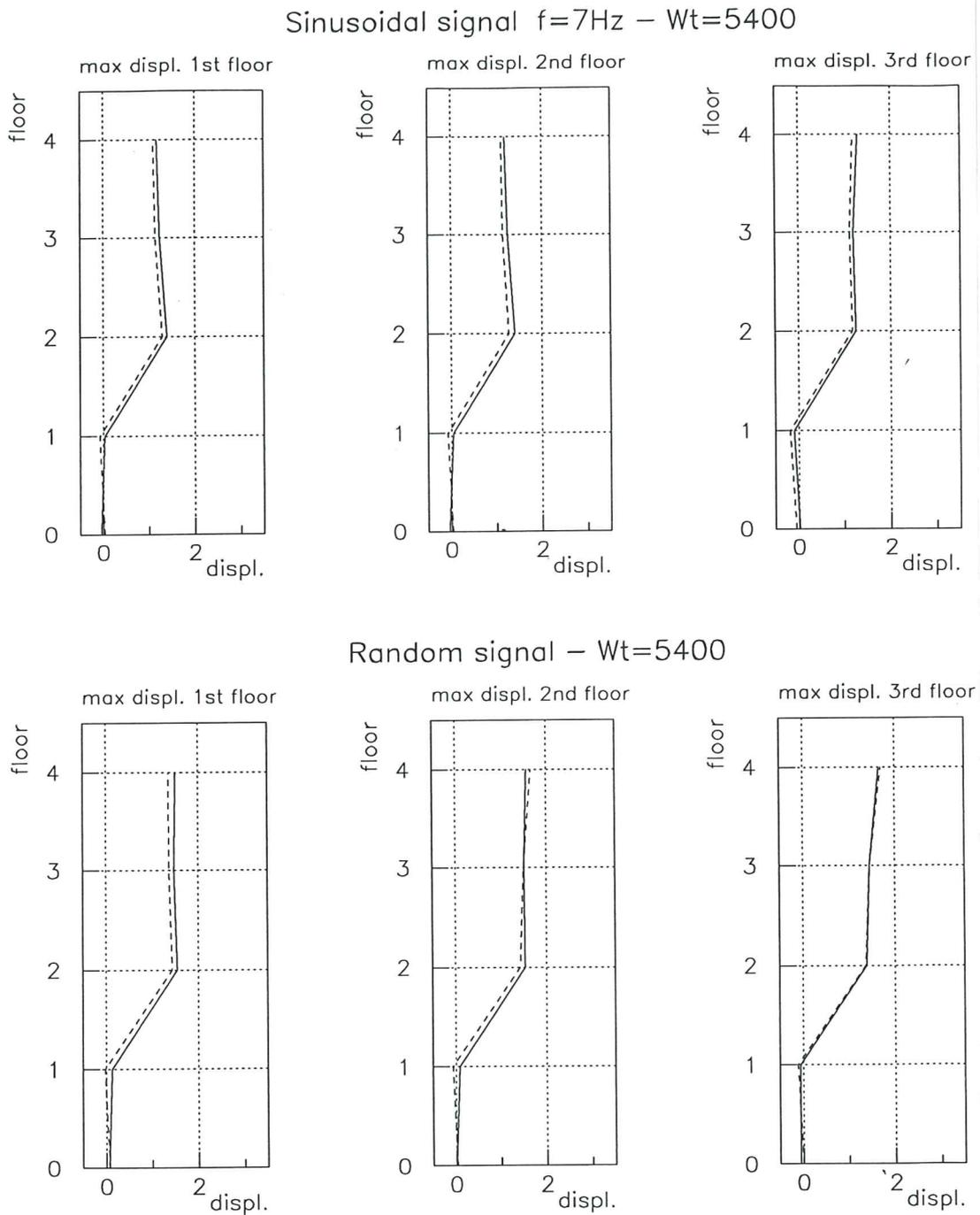
**Fig. 29b.** Deflected shape at maximum story displacements for a sinusoidal signal ( $f=7\text{Hz}$ ) and a random signal.
