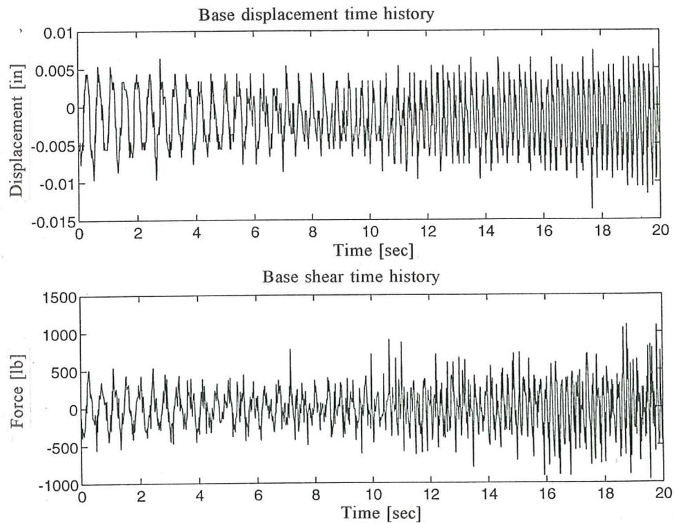
**Fig. 31d.** Base displacement time history and base shear time history for the fixed base model subjected to a sweep frequency signal. Range [2000 3000].
