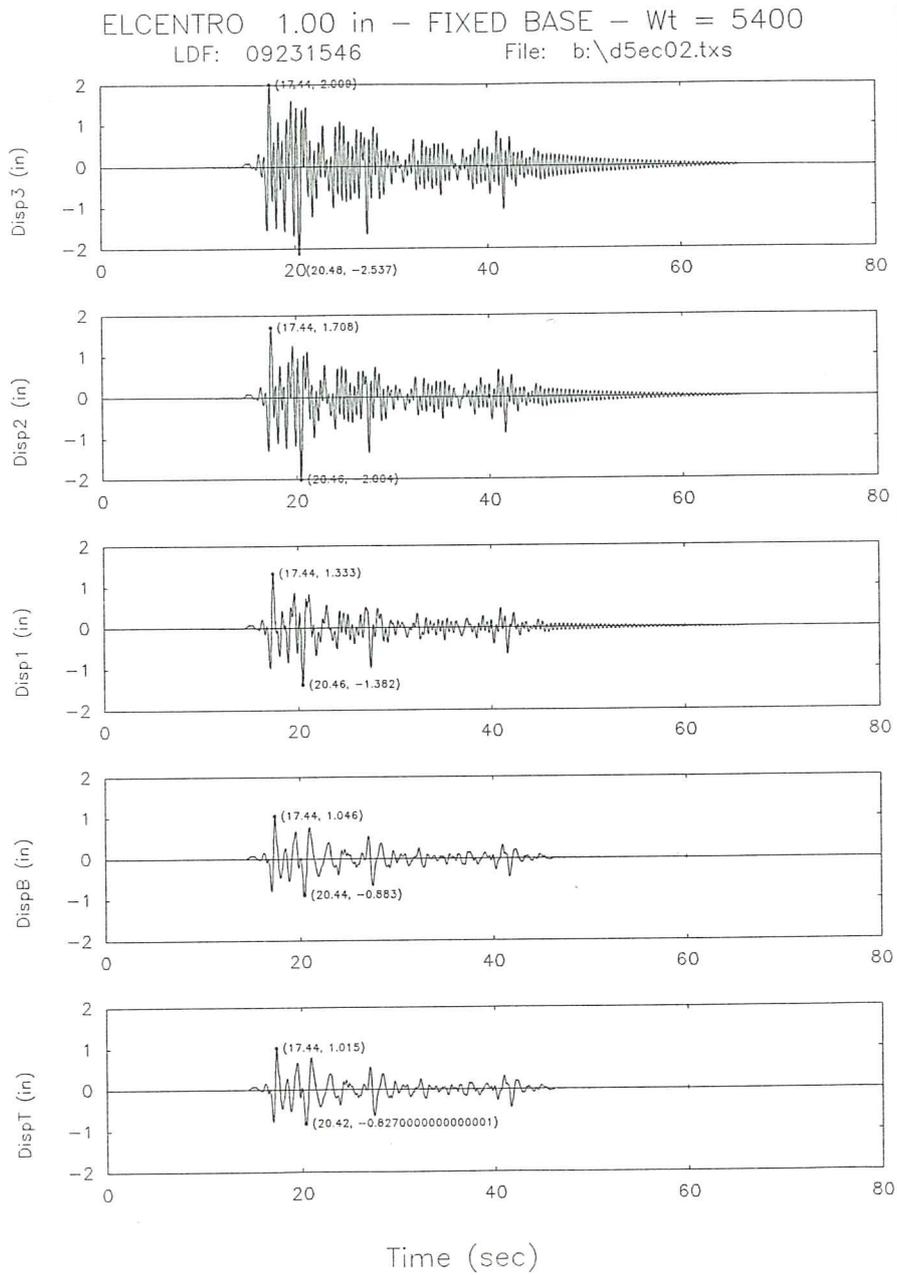
Fig. 24c. Displacement time responses for the fixed base model subjected to El Centro signal.
