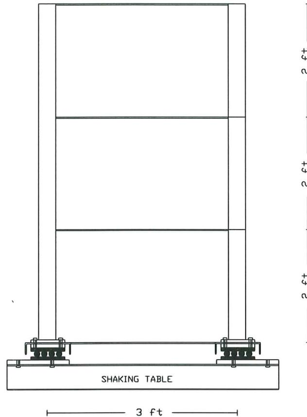
Fig. 6. The base isolated model
