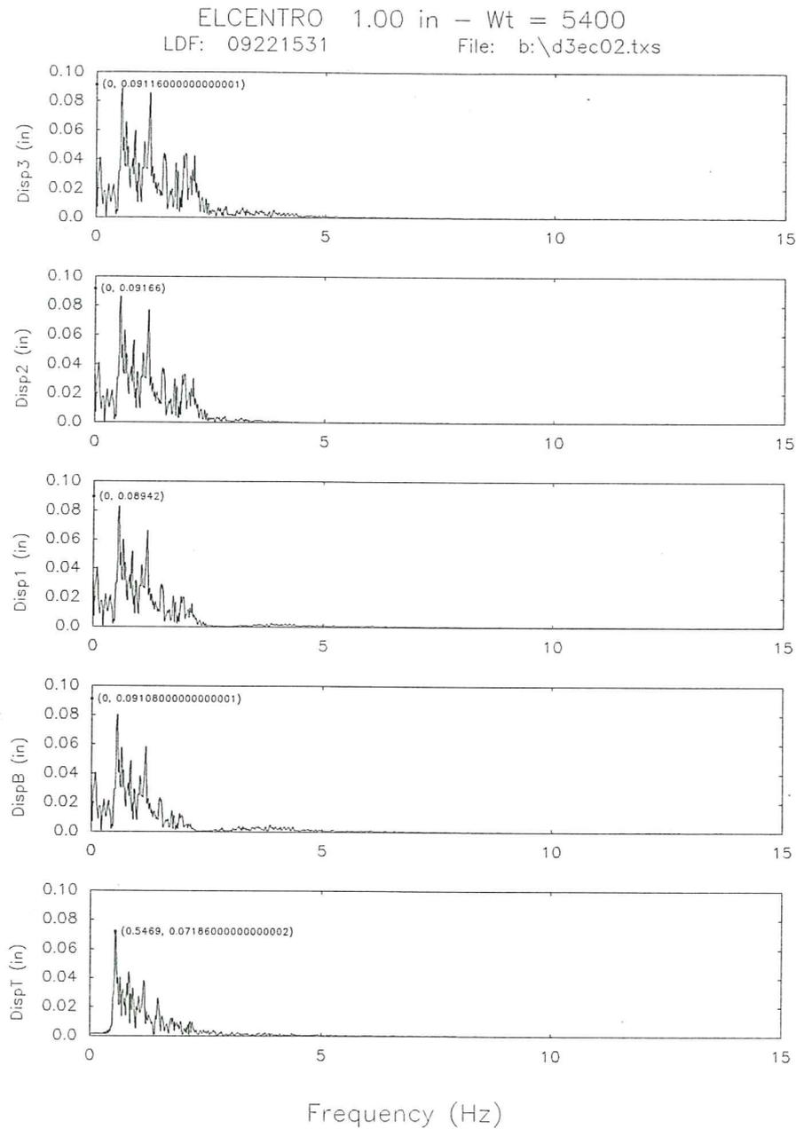
**Fig. 23d.** Fourier spectra of the displacements for the base isolated model subjected to El Centro signal.
