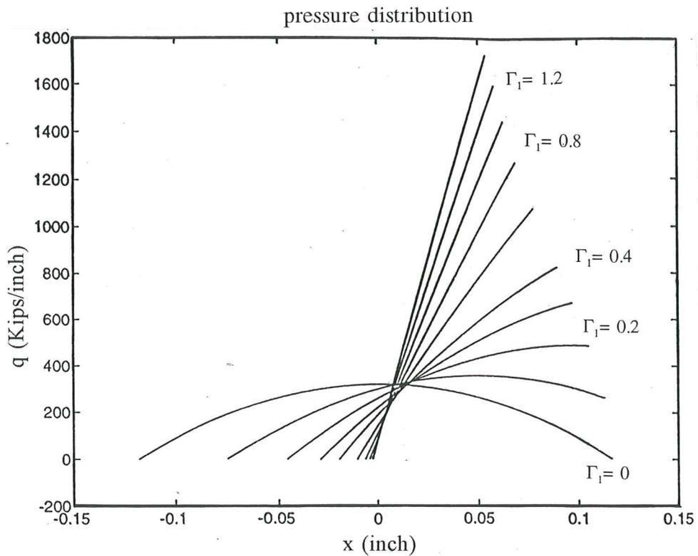
Fig. 4. Pressure distribution under a vertical load  $Q=50$  pounds, for different values of  $\Gamma_1$ .
