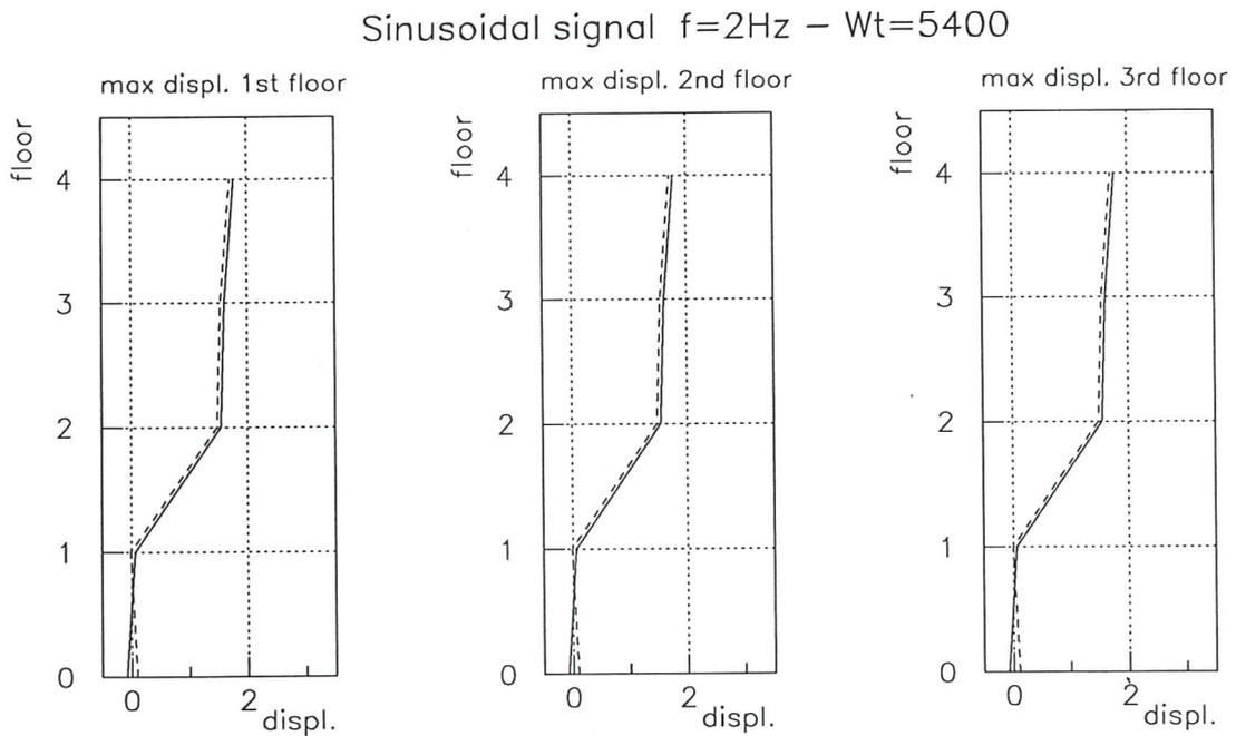
**Fig. 29a.** Deflected shape at maximum story displacements for a sweep frequency signal and a sinusoidal signal.
