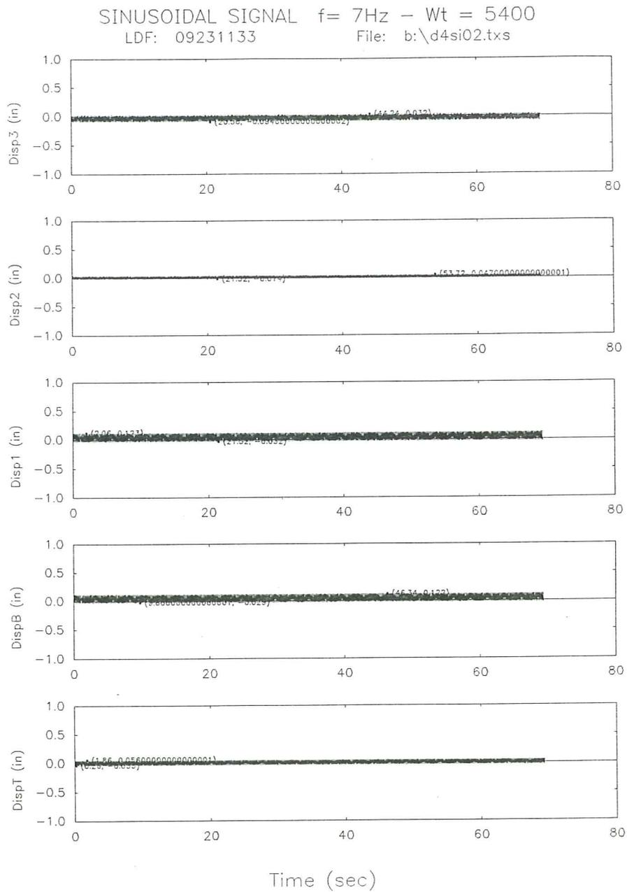
Fig. 20c. Displacement time responses for the base isolated model subjected to a sinusoidal signal ( $f=7\text{Hz}$ ).
