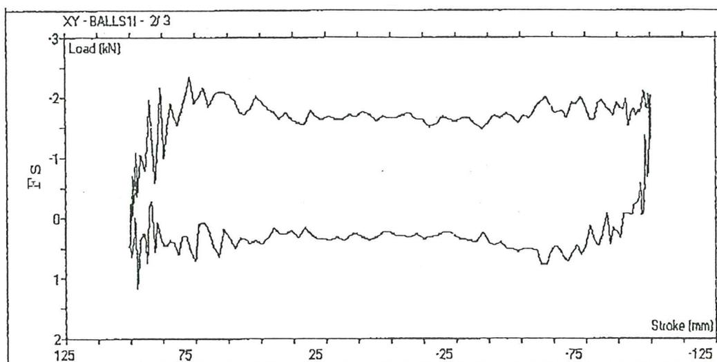
Fig. 12b. Exp.1. 2nd loop of 5 loops - sinewave of 0.1 Hz  $\pm$  100mm.
