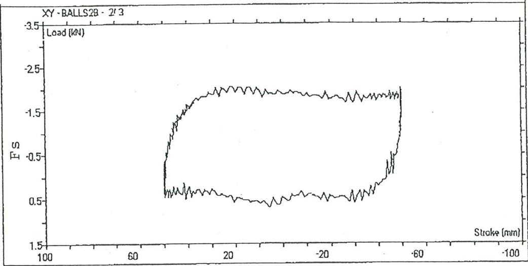
Fig. 11b. Exp.1. 2nd loop of 5 loops - sinewave of 0.5 Hz ± 50mm.
