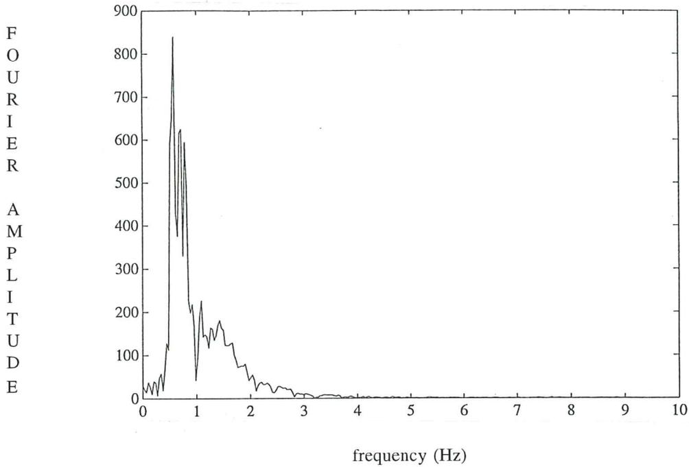
Fig. 13c. Fourier spectra. Parkfield 1966, N65 component.
