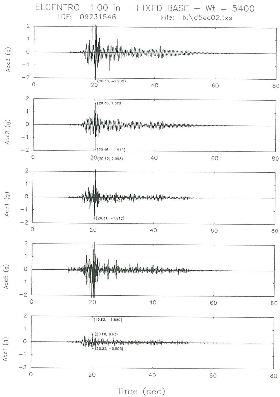
Fig. 24a. Acceleration time response for the fixed base model subjected to El Centro signal.
