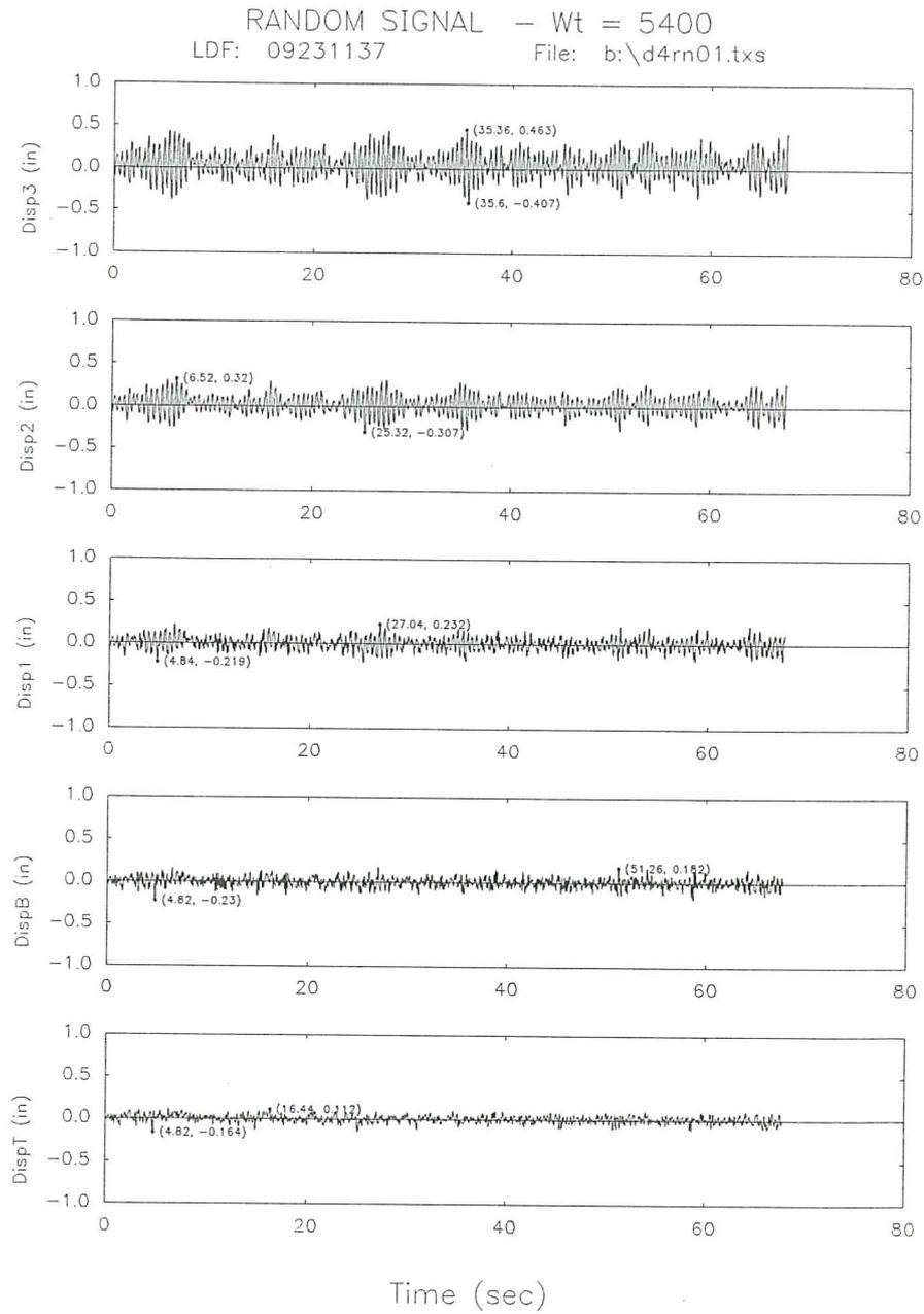
Fig. 16c. Displacement time responses for the base isolated model subjected to a random signal.
