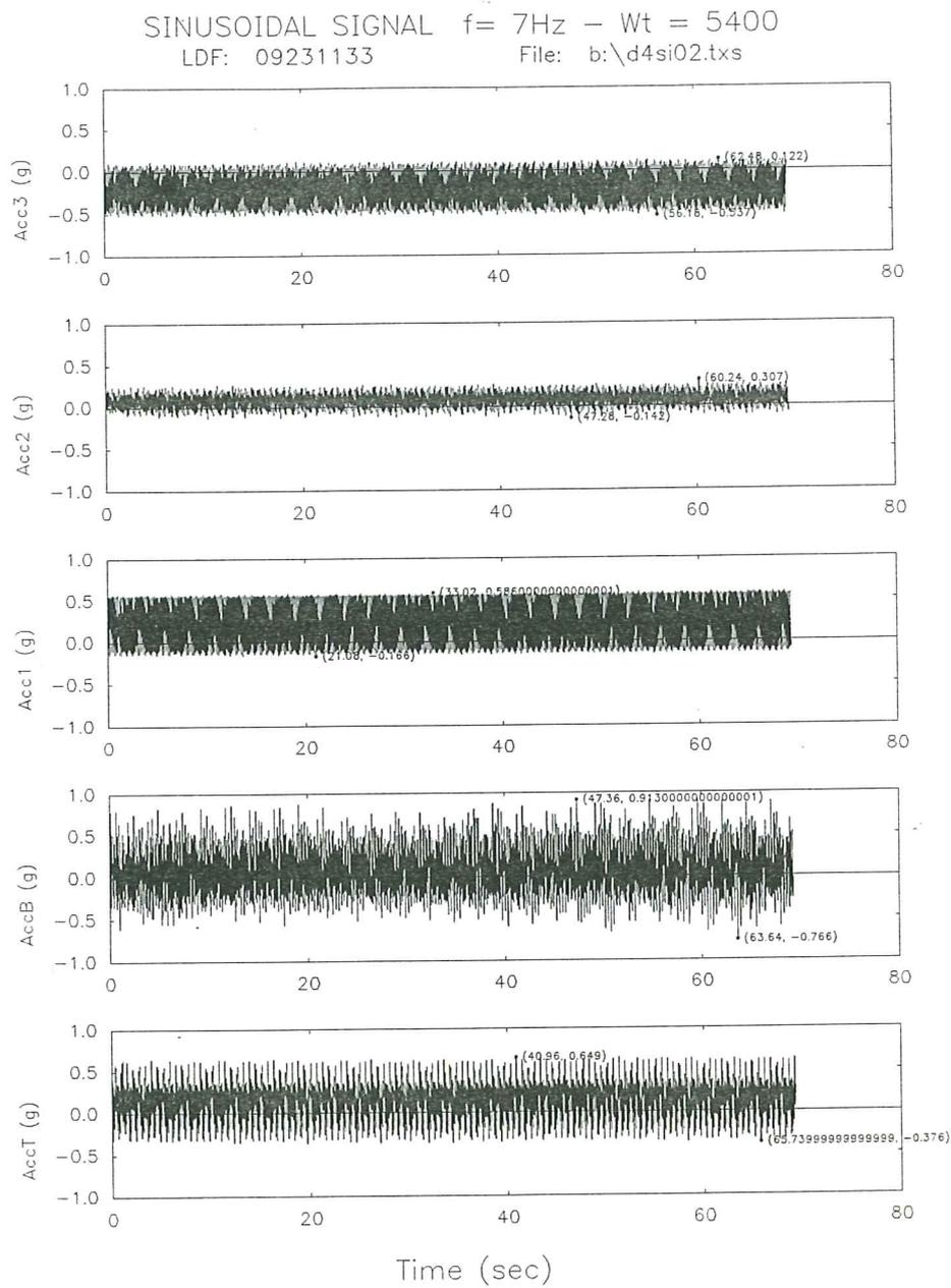
Fig. 20a. Acceleration time response for the base isolated model subjected to a sinusoidal signal ( $f=7\text{Hz}$ ).
