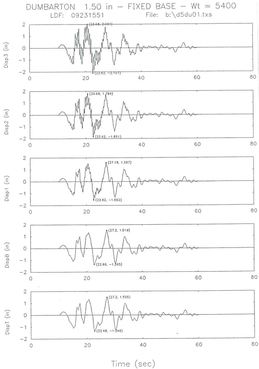
Fig. 28c. Displacement time responses for the fixed base model subjected to Dumbarton signal.
