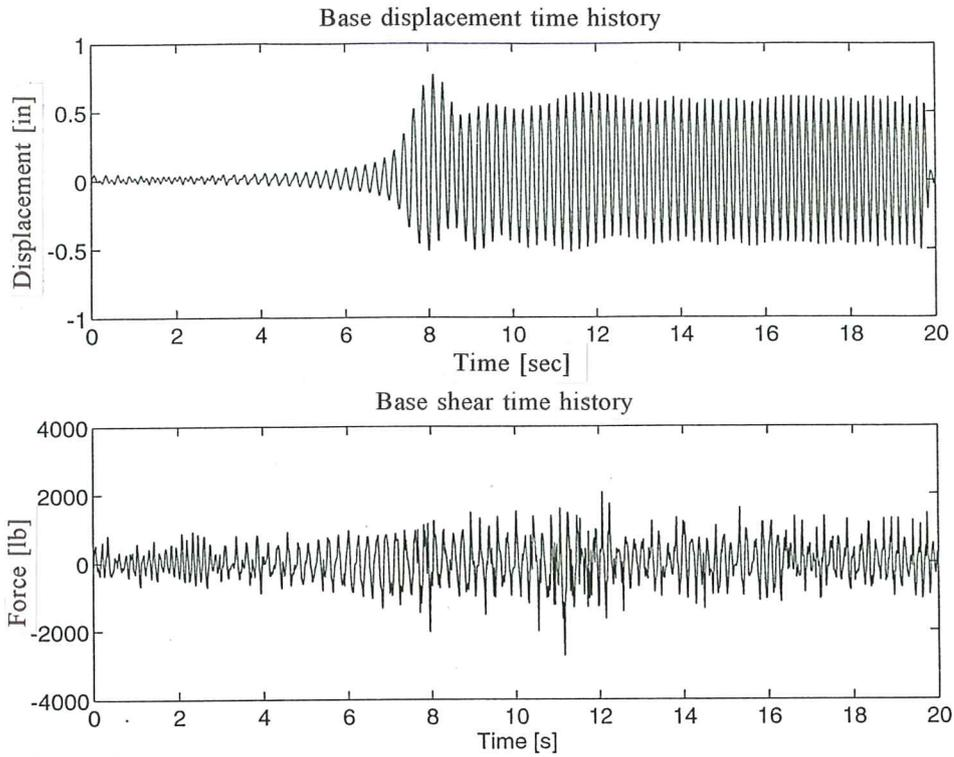
**Fig. 31a.** Base displacement time history and base shear time history for the base isolated model subjected to a sweep frequency signal. Range [1000 2000].
