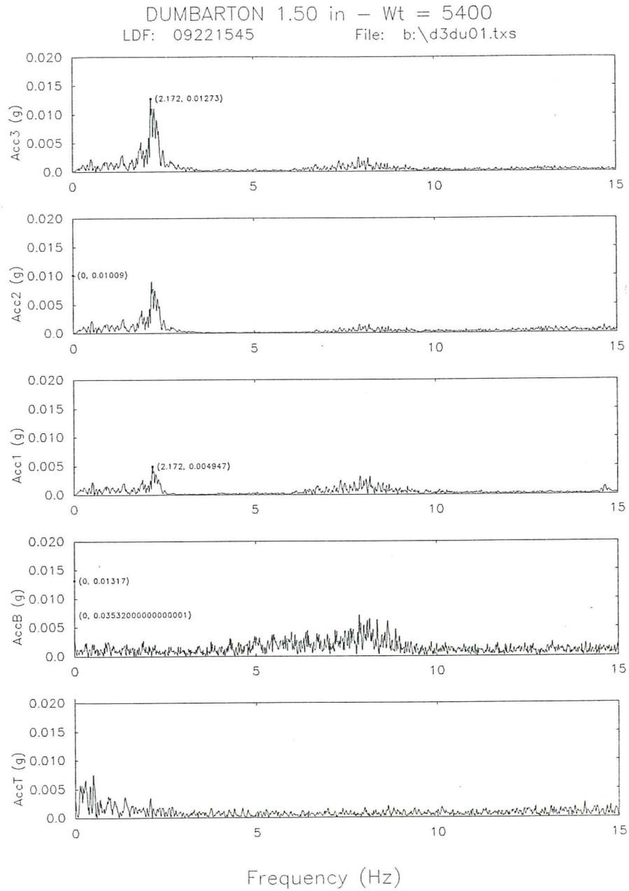
Fig. 27b. Fourier spectra of the accelerations for the base isolated model subjected to Dumbarton signal.
