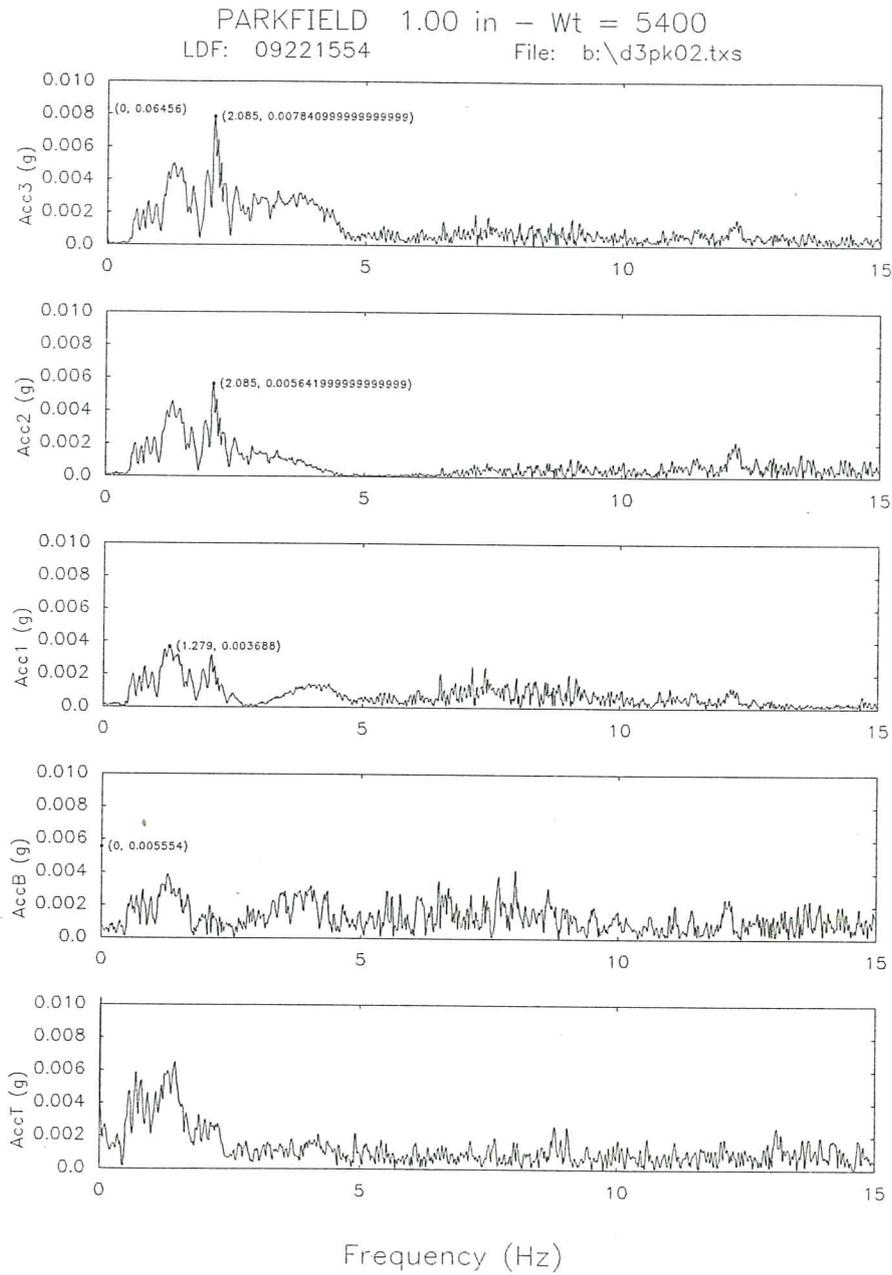
**Fig. 25b.** Fourier spectra of the accelerations for the base isolated model subjected to Parkfield signal.
