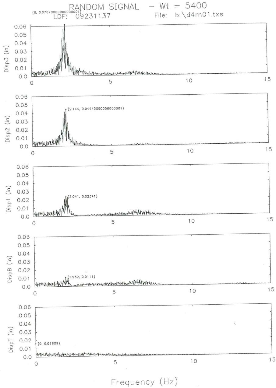
Fig. 16d. Fourier spectra of the displacements for the base isolated model subjected to a random signal.
