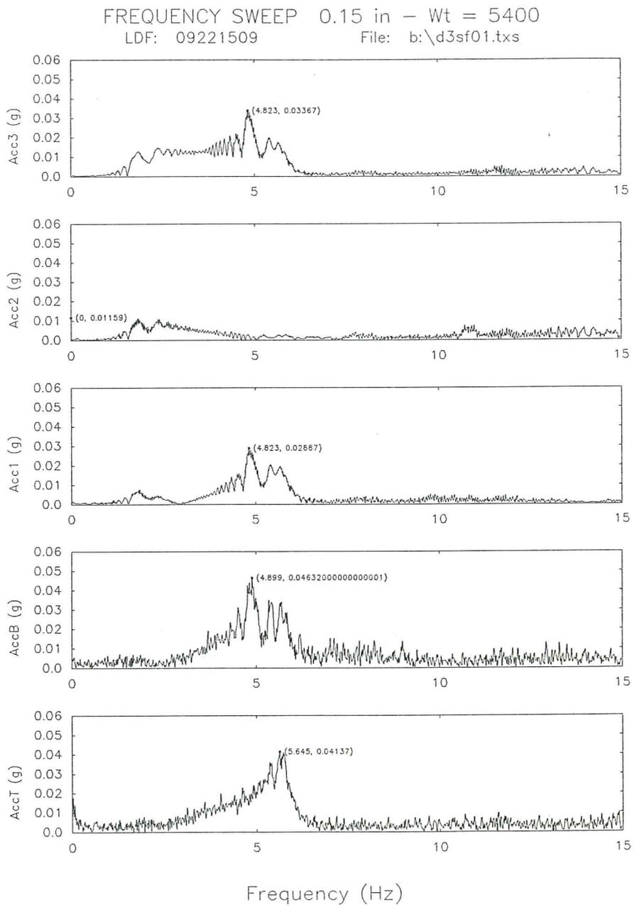
Fig. 14b. Fourier spectra of the accelerations for the base isolated model subjected to a sweep frequency signal.
