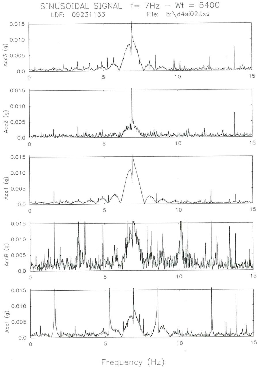
**Fig. 20b.** Fourier spectra of the accelerations for the base isolated model subjected to a sinusoidal signal ( $f=7\text{Hz}$ ).
