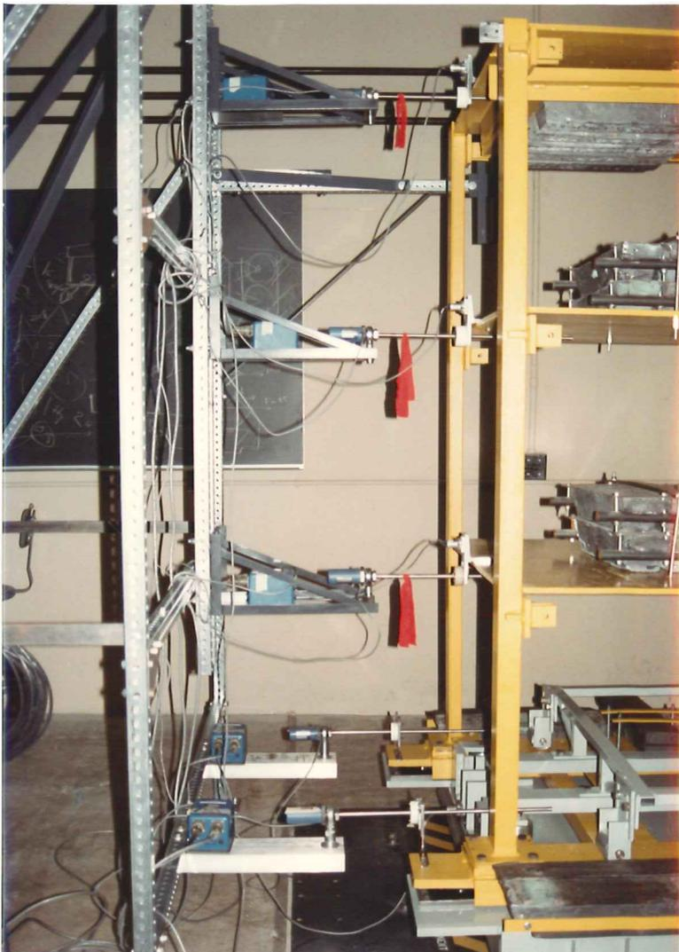
**Photo 6.** Accelerometers and displacement transducers.
