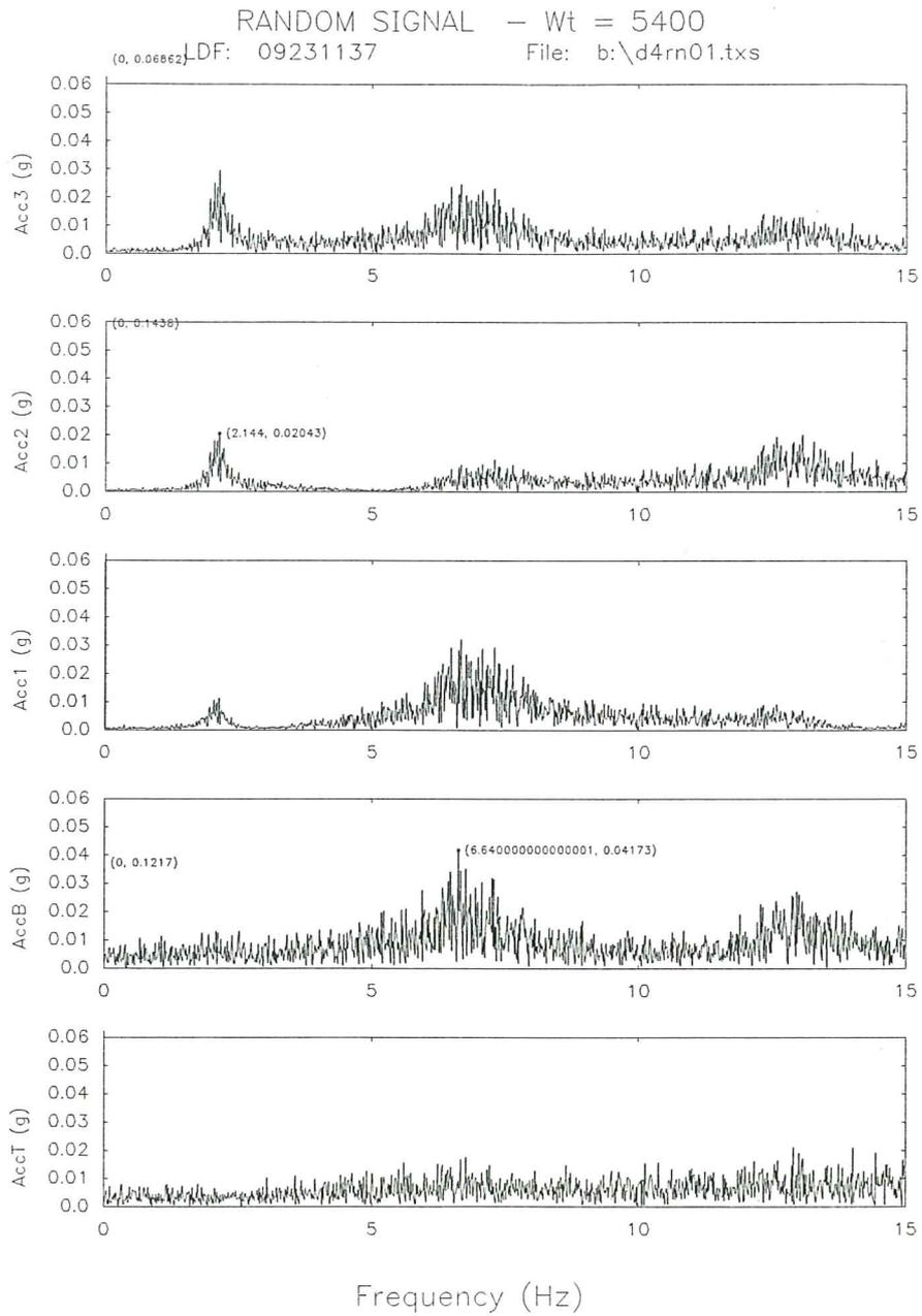
**Fig. 16b.** Fourier spectra of the accelerations for the base isolated model subjected to a random signal.
