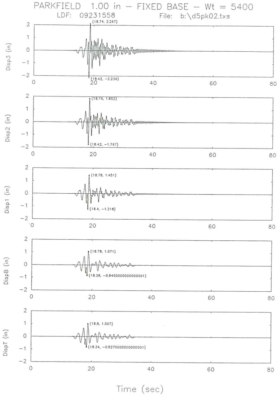
Fig. 26c. Displacement time responses for the fixed base model subjected to Parkfield signal.
