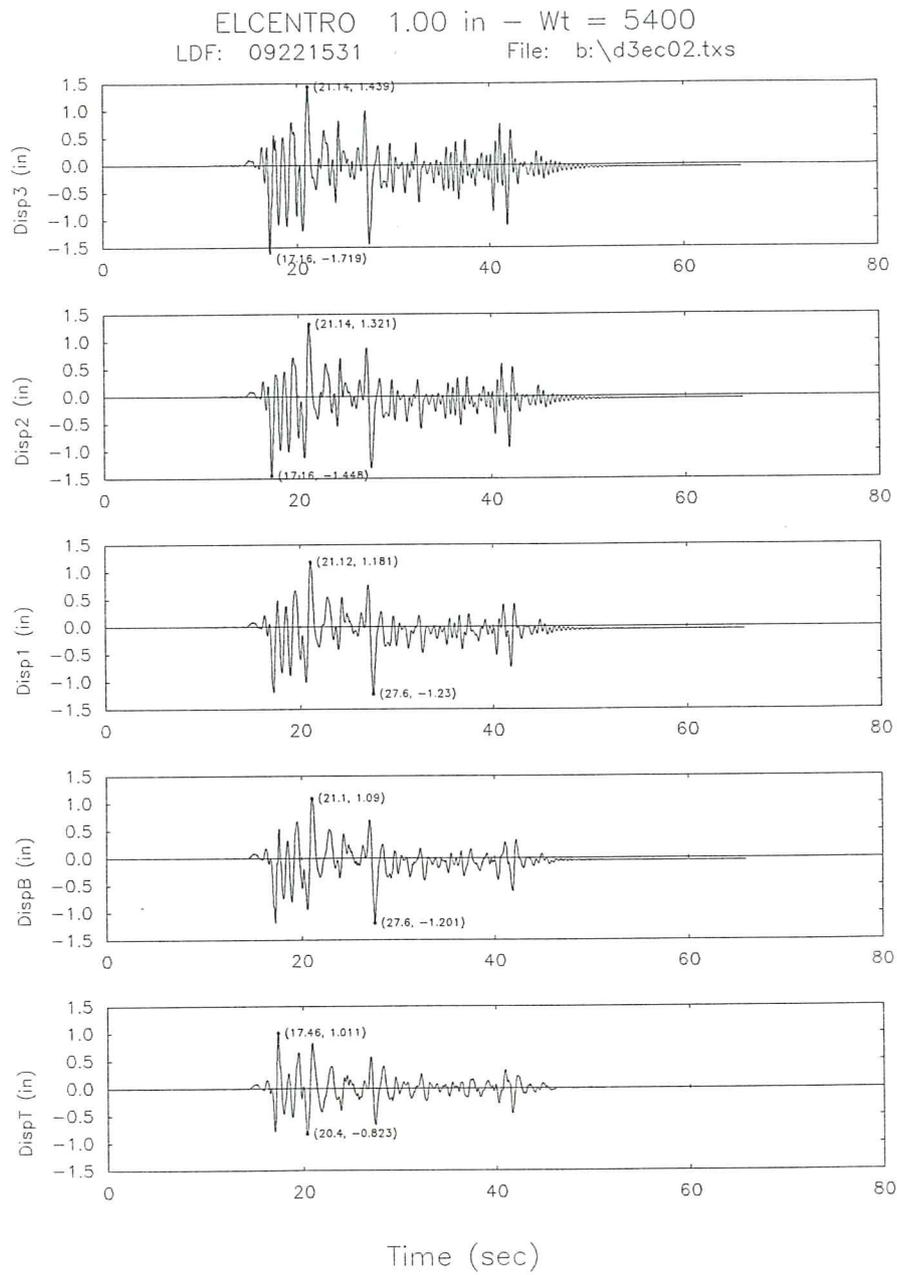
Fig. 23c. Displacement time responses for the base isolated model subjected to El Centro signal.
