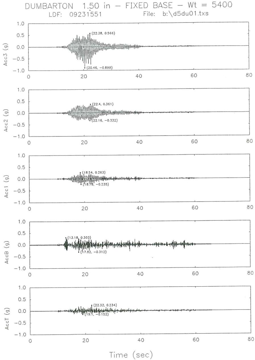
Fig. 28a. Acceleration time response for the fixed base model subjected to Dumbarton signal.
