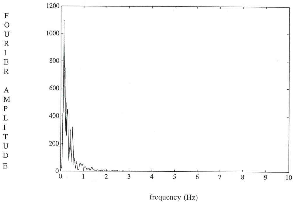
Fig. 13b. Fourier spectra. Dumbarton 1989, 267 Degrees.
