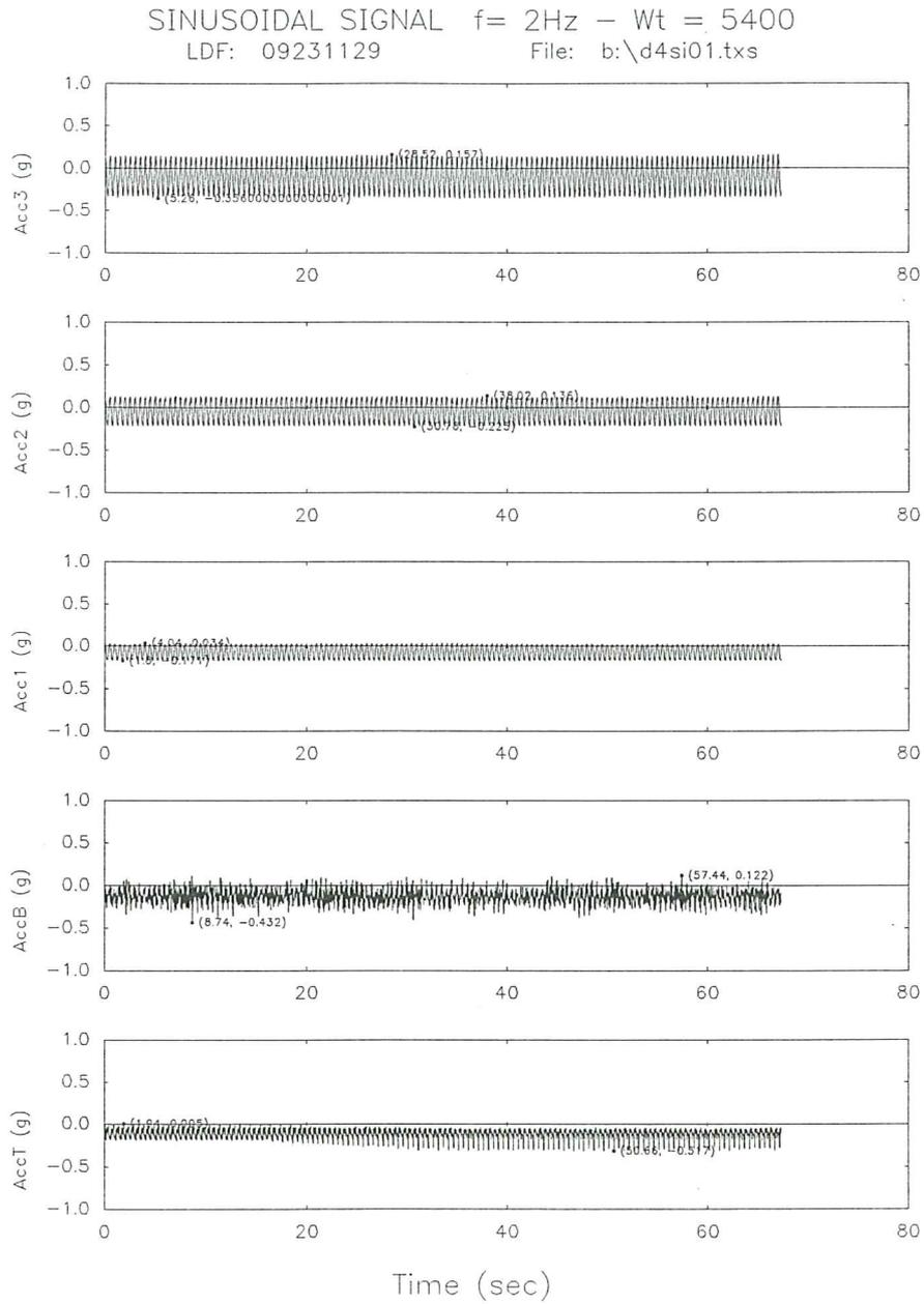
Fig. 18a. Acceleration time response for the base isolated model subjected to a sinusoidal signal ( $f=2\text{Hz}$ ).
