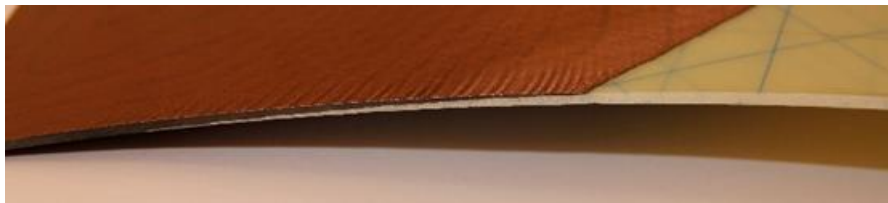
Figure1: Cross-section of scarfed GFRP “window” (flare) of the winglet
