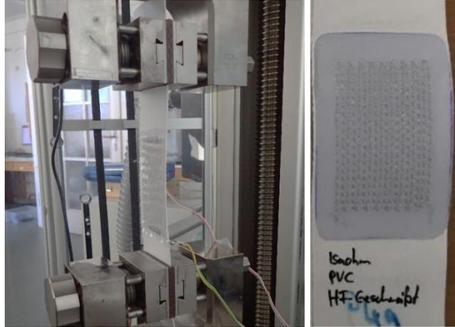
Figure 6: Uniaxial tensile test – sensor concept 1
