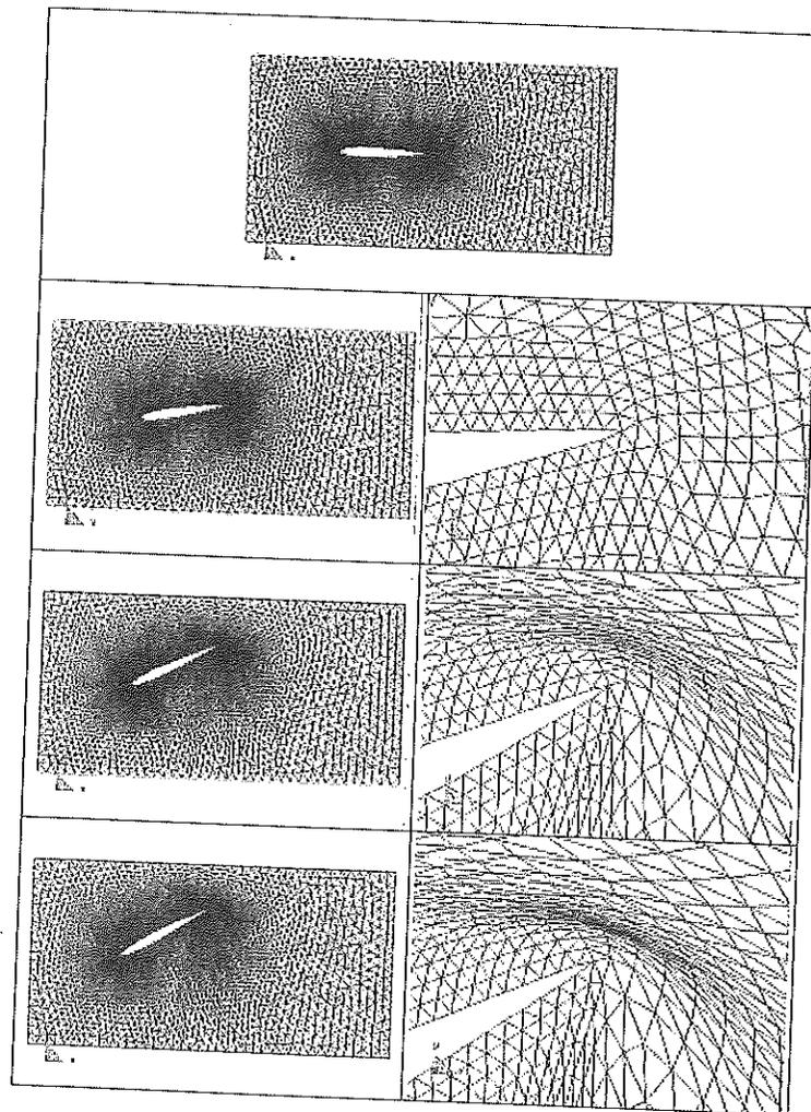
Figure 2: Original NACA0012 airfoil discrete model (first row). Tail vertical displacement of the airfoil using a Young modulus distribution depending quadratically on the distance from the elements to the moving surfaces (strategy 4). The 18% and the 50% chord length displacement are shown in the second and third row respectively. The maximum tail vertical displacement before element intersection has been about 55% of the chord length and is shown (fourth row).
