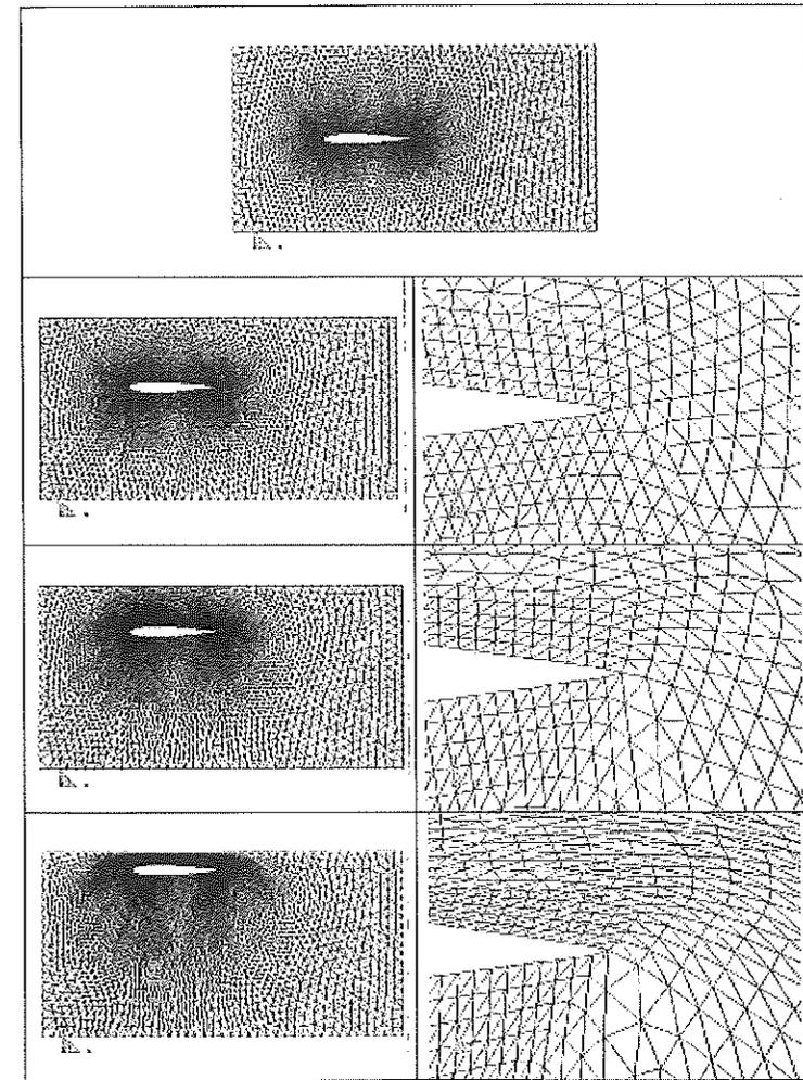
Figure 9: Original NACA0012 airfoil discrete model (first row). Vertical change of position of the airfoil using a Young modulus distribution depending on the square norm of the principal strains (strategy 8). The 24% and 50% chord length displacement is shown in the second and third row respectively. The maximum vertical change of position before element intersection has been about 81% of the chord length (fourth row).
