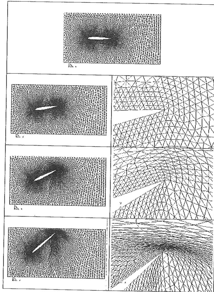
Figure 8: Original NACA0012 airfoil discrete model (first row). Tail vertical displacement of the airfoil using a Young modulus distribution depending on the square norm of the principal strains (strategy 8). The 18% and 50% chord length displacement are shown in the second and third row respectively. The maximum tail vertical displacement before element intersection has been about 87% of the chord length (fourth row).
