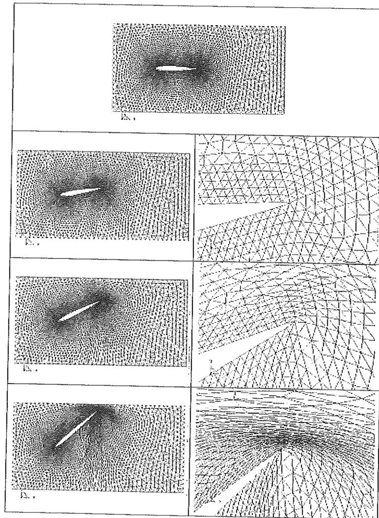
Figure 6: Original NACA0012 airfoil discrete model (first row). Tail vertical displacement of the airfoil using a Young modulus distribution proportional to the distortion energy density of the elements (strategy 7). The 18% and 50% chord length displacement are shown in the second and third row respectively. The maximum tail vertical displacement before element intersection has been about 82% of the chord length (fourth row).
