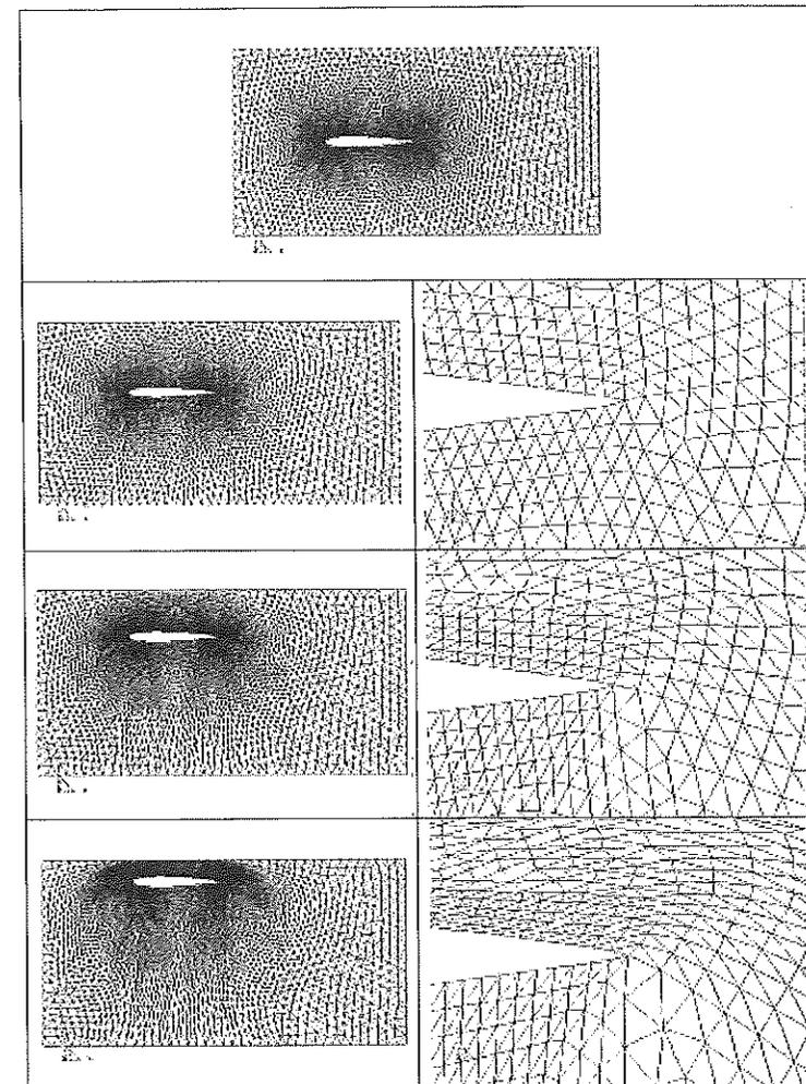
Figure 7: Original NACA0012 airfoil discrete model (first row). Vertical change of position of the airfoil using a Young modulus distribution proportional to the distortion energy density of the elements (strategy 7). The 24% and 50% chord length displacement are shown in the second and third row respectively. The maximum vertical change of position before element intersection has been about 80% of the chord length (fourth row).
