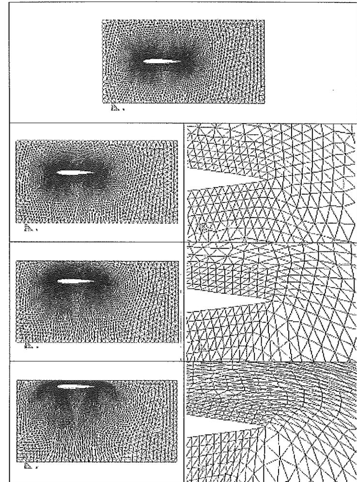
Figure 5: Original NACA0012 airfoil discrete model (first row). Vertical change of position of the airfoil using a Young modulus distribution depending on the strain energy density of the elements (strategy 6). The 24% and 50% chord length displacement are shown in the second and third row respectively. The maximum vertical change of position before element intersection has been about 85% of the chord length (fourth row).
