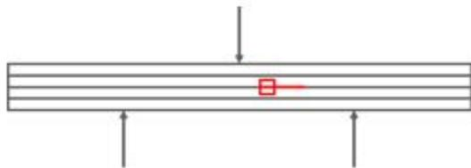
Midplane crack at 0° and 90° interface
