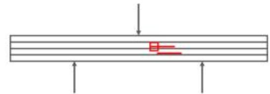
Intraply crack in second ply and interply crack between third and fourth plies from top at fibre-matrix interface
