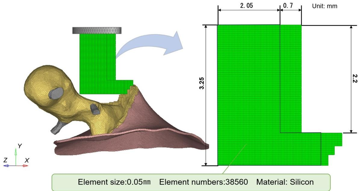
**Figure 8:** Design domain for the application example in the type-IV tympanoplasty operation
