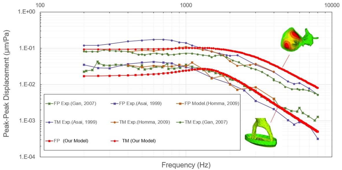
**Figure 7:** Comparison of harmonic vibration analysis results with reference measurement values
