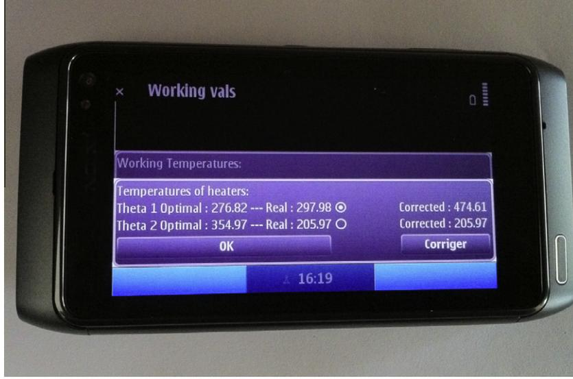
Fig. 12. System reconfiguration by adjusting the temperature of the first heating device.
