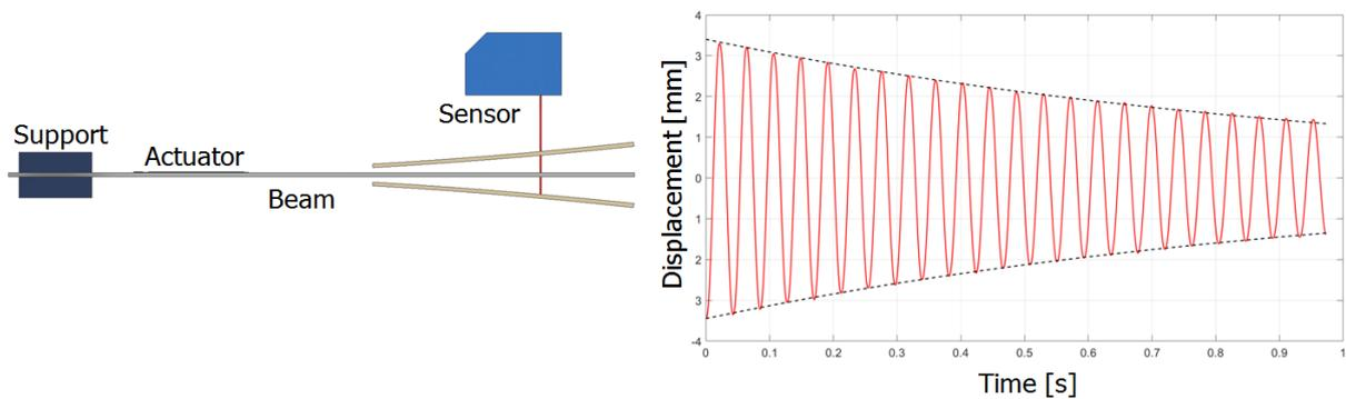
Figure 4: Free vibration test: 1<sup>st</sup> bending vibration mode
