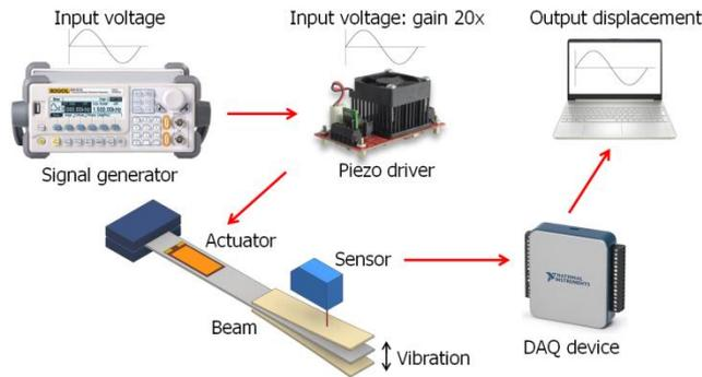
**Figure 2:** The experimental setup scheme
