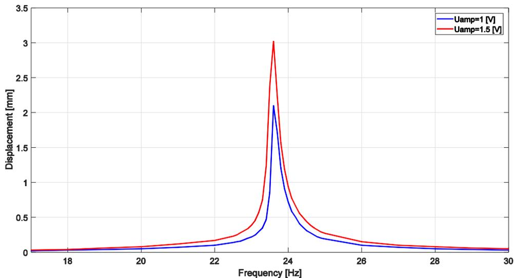
**Figure 5:** Forced vibration test: displacement amplitude-frequency characteristics
