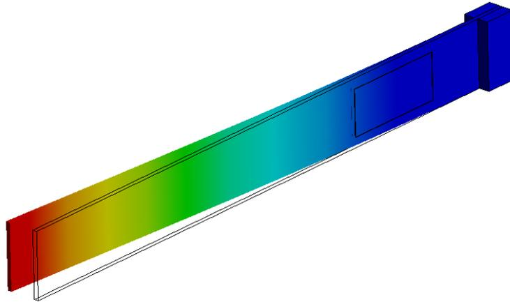
**Figure 7:** Modal analysis: beam's 1<sup>st</sup> vibration mode at 23.64 Hz
