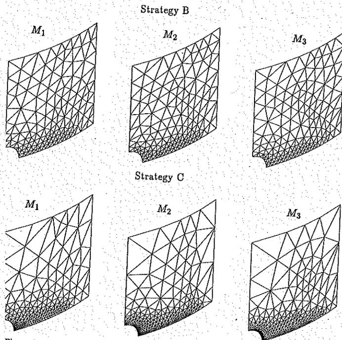
Figure 3. Analysis of a cylindrical shell under uniform traction. Sequence of meshes obtained with AMR strategies based on: Equal distribution of global error (Strategy B) and Equal distribution of specific error (Strategy C).
