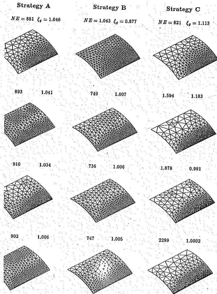
Figure 2. Symmetric quadrant of a cylindrical shell roof under self weight. Sequence of meshes obtained with AMR strategies based on: (A) Equal distribution of global error and inconsistent definition of parameter  $\xi$  (viz eq.(17)); (B) Idem with  $\xi$  consistently defined by eq.(16); and (C) Equal distribution of specific error. For each mesh is shown the number of elements (NE) and the value of the global error parameter  $\xi_g$ .
