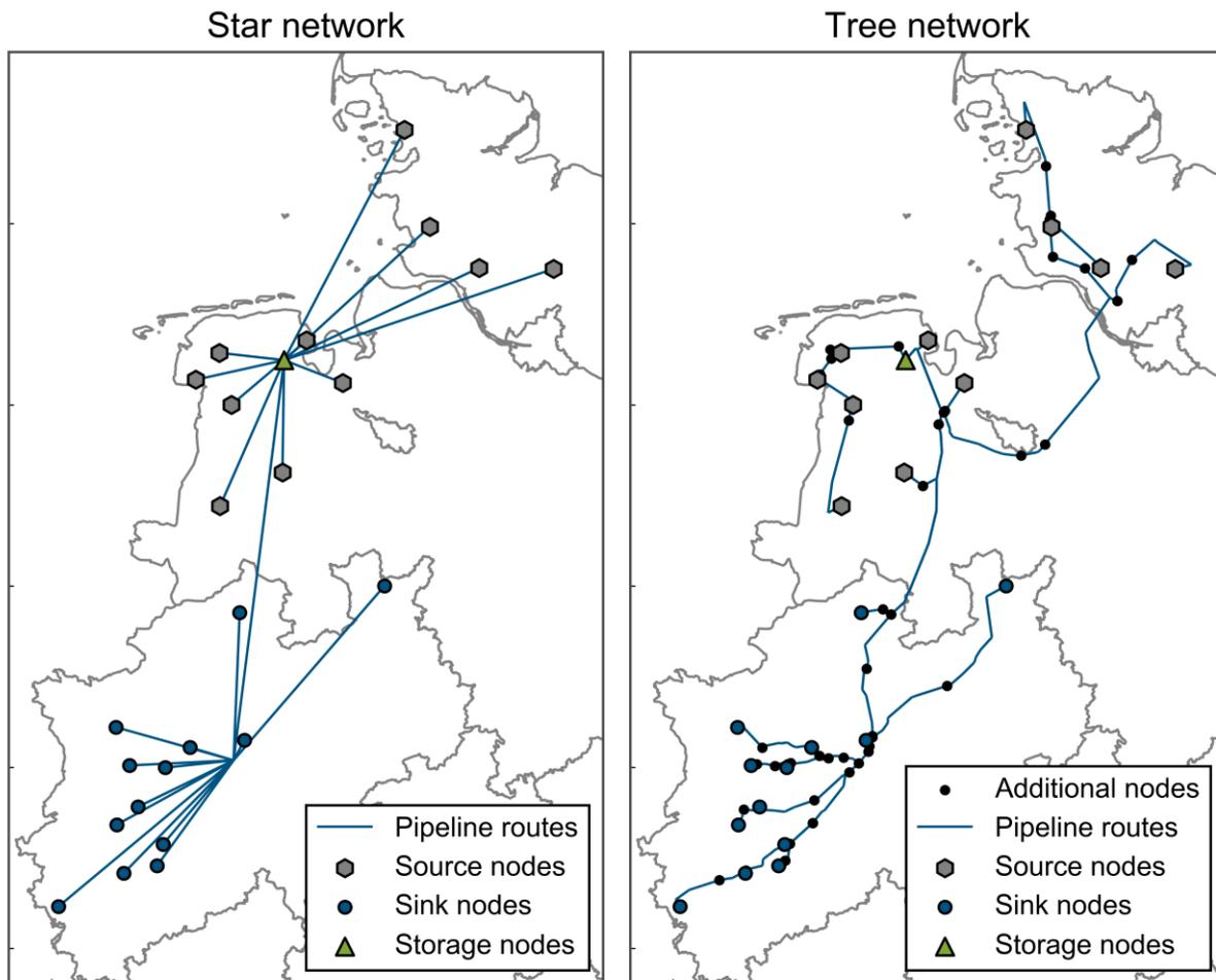
**Figure 6. Model view on the pipeline network. Left: star network with connections from electrolysis to storage, from storage to the centroid of NRW, and from the centroid of NRW to power plant locations. Right: tree network with a fine pipeline grid.**
