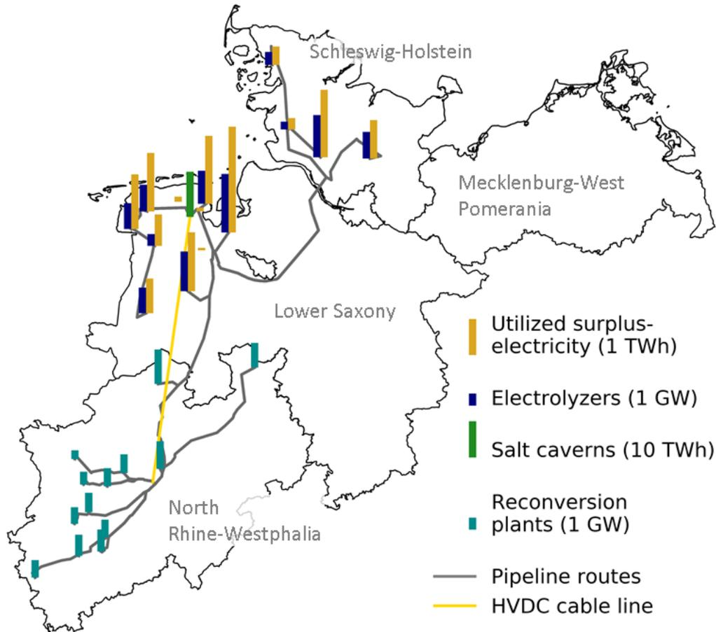
**Figure 5. Installed capacities of the CCGT reconversion power plants, storage capacity of the salt caverns, surplus electricity used, and the pipeline routes, as well as HVDC routes in the cost-optimized reconversion pathway, reproduction from Welder et al. [11], with permission from Elsevier.**
