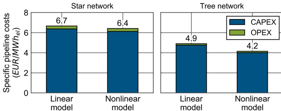
**Figure 15. Comparison of specific pipeline costs for two different networks and two different flow modelling approaches. Total re-electrification costs from Welder et al. [11] for the CCGT scenario are 176 EUR/MWh<sub>el</sub>.**
