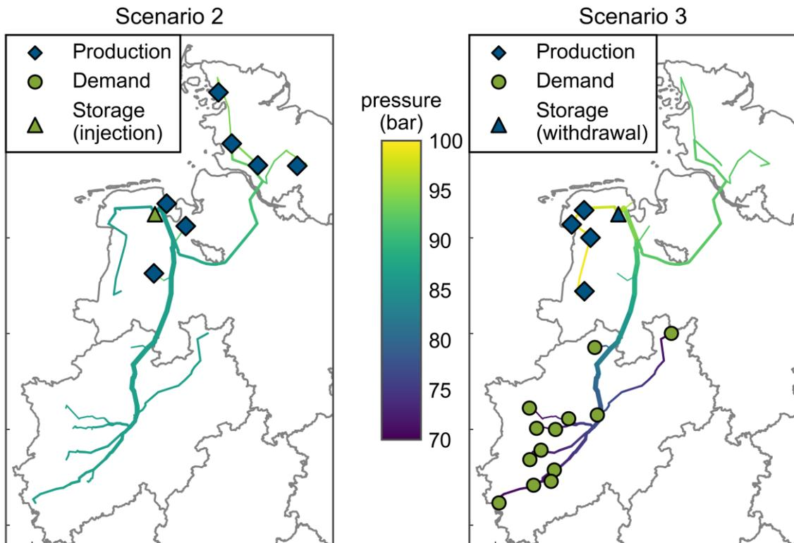
Figure 12. Exemplary pressure gradients of the tree network for scenario 2 (lowest pressure gradient) and scenario 3 (largest pressure gradient).
