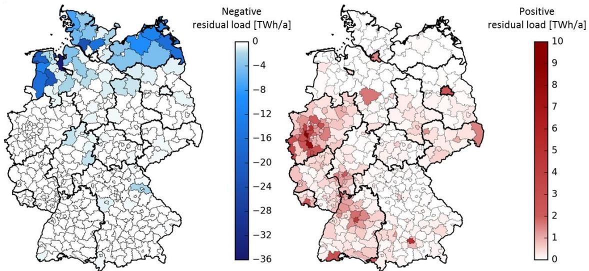
**Figure 3: Negative (blue) and positive (red) residual load for Germany in 2050 based on the electricity system assumptions from Robinius et al. [35], reproduction from Emonts et al. [36], with permission from Elsevier.**
