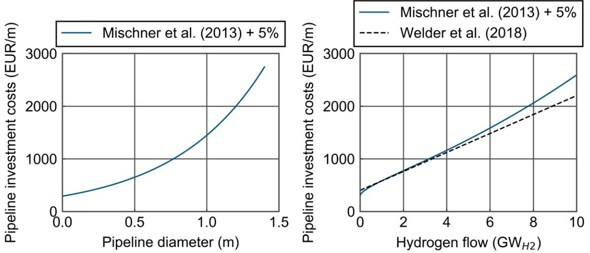
**Figure 2. Left: pipeline investment costs dependent on pipeline diameter according to Mischner et al. [33]; right: adjusted pipeline investment costs from Mischner et al. [33], Equation (2), for gas velocity (10 m/s) and density (5.7 kg<sub>H2</sub>/m<sup>3</sup>) compared to the linearized cost function from Welder et al. [11], Equation (3), depending on the maximum flow.**
